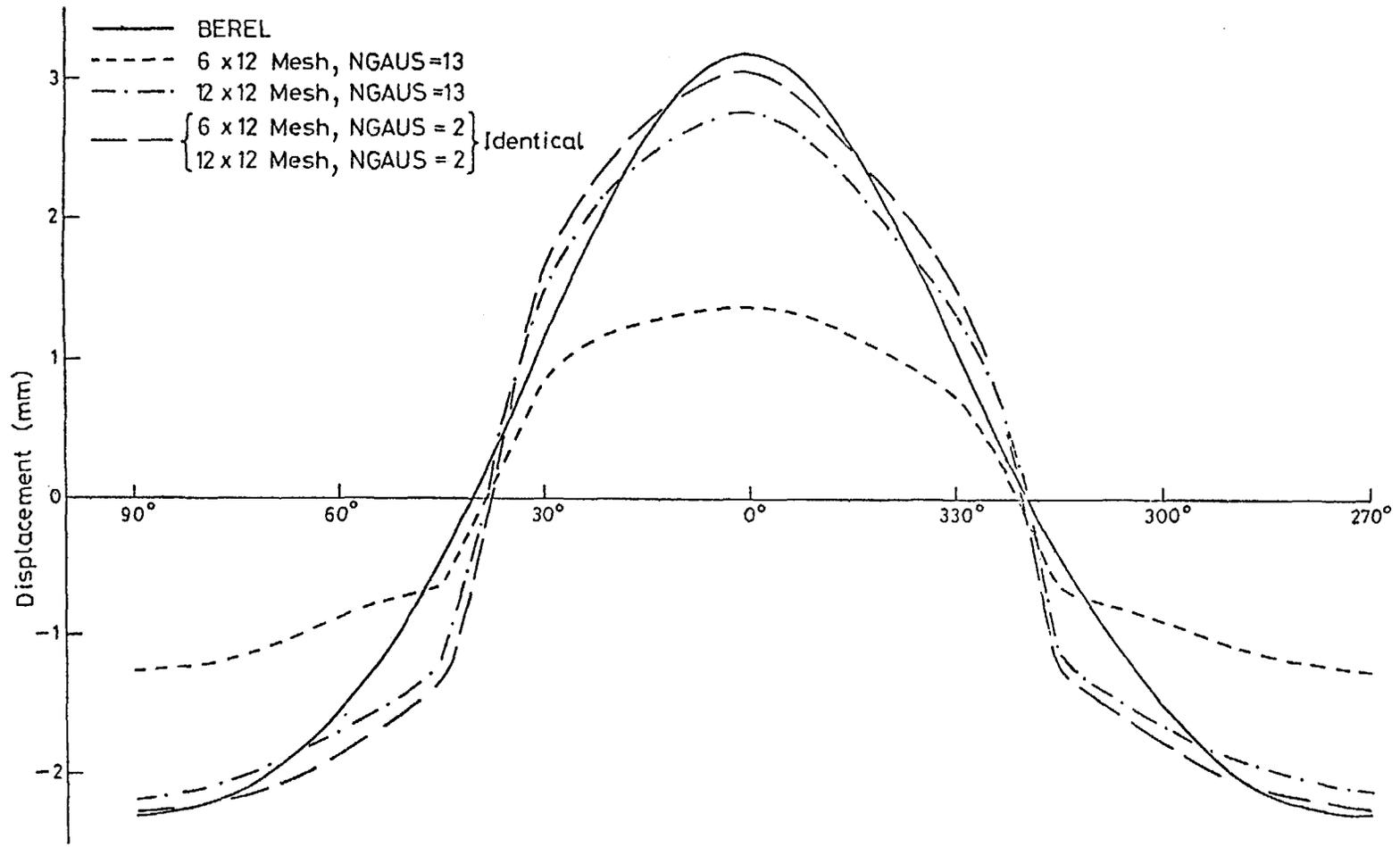
FIG. 6. Radial Displacements Around Outside Surface in Symmetry Plane X=0 for Brick Elements. Load = 61000N, Elastic Conditions.
