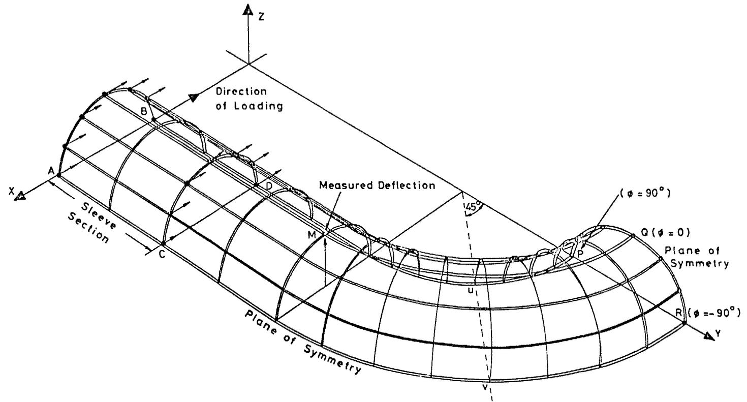
**FIG. 2** Finite Element Discretization of Pipe Bend (Medium Mesh)
