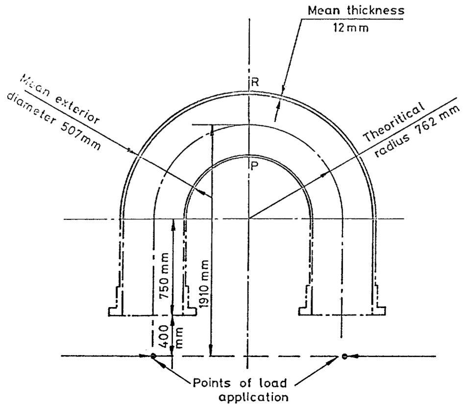
FIG.1.      Geometry of Pipe Bend.
