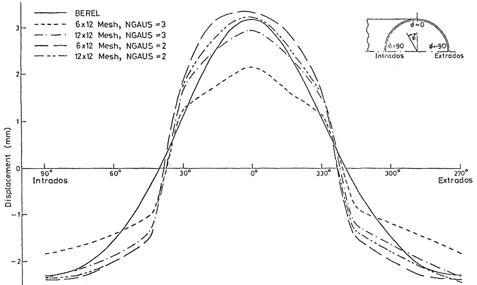
FIG.7. Radial Displacements Around Mid Surface in Symmetry Plane  $X=0$  for Loof Elements. Load = 61000 N, Elastic Conditions.
