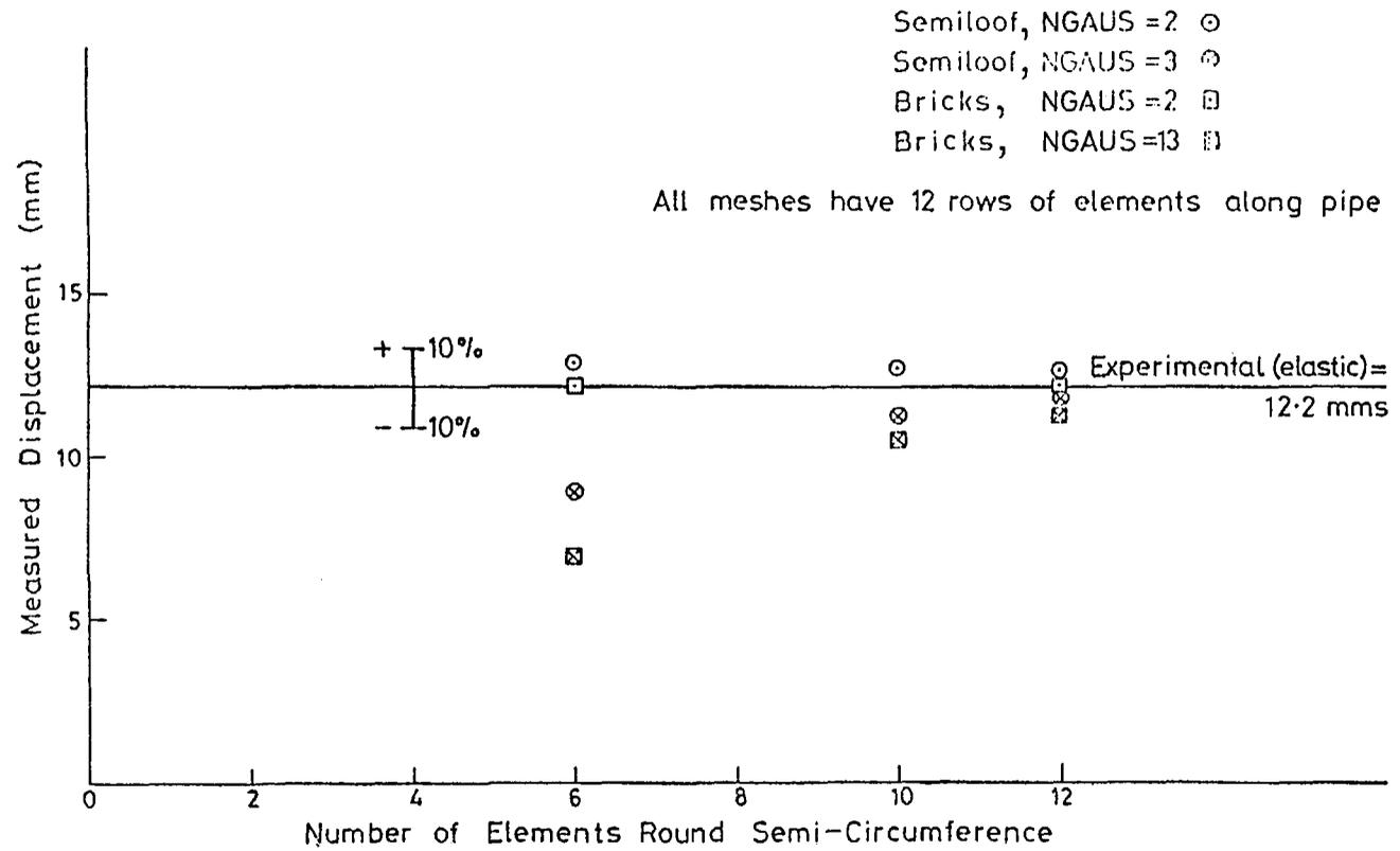
FIG.5. Measured Point Displacements for Different Meshes, Elements and NGAUS.
