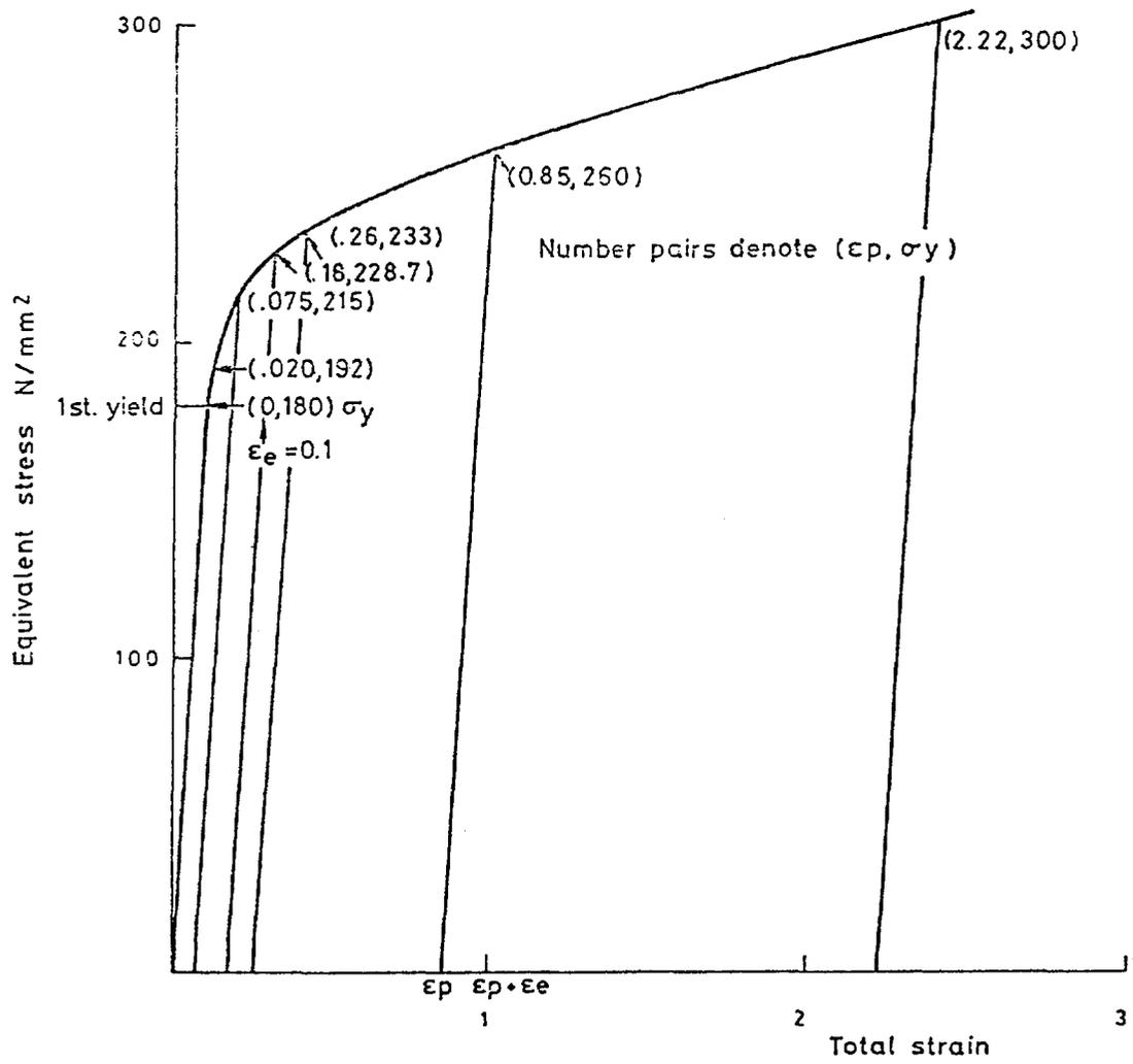
FIG.4. Non-Linear Data for Pipe Bend.
