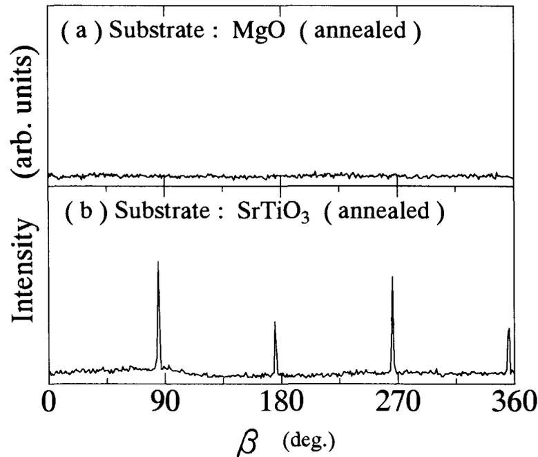
**Figure 5** Intensity change of the (102) reflection due to  $\beta$  scan for Y-123 on (a) MgO and (b) SrTiO<sub>3</sub>.
