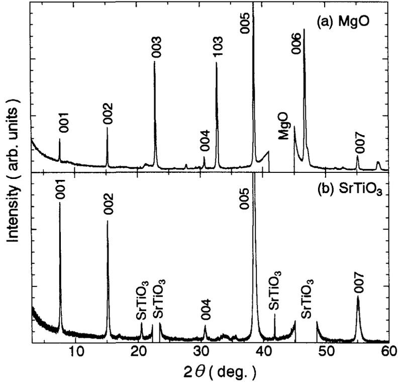
**Figure 4** XRD patterns of the Y-123 thin films on (a) MgO and (b) SrTiO<sub>3</sub>.
