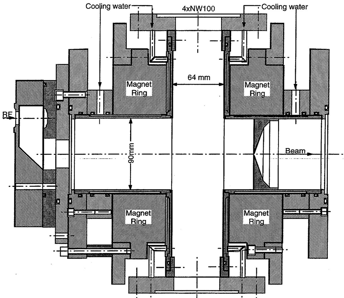
**Figure 2: schematic drawing of the mono1001. A target can be mounted on one of the 64 mm inner diameter flange.**
