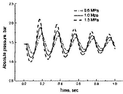
Fig. 9 The effect of driving steam pressure on the bubble pressure history.
