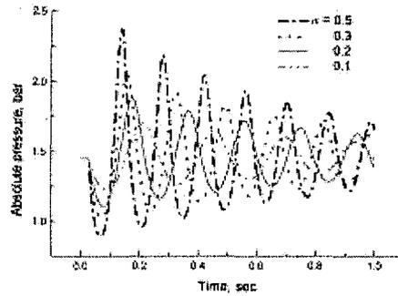
Fig. 12 The effect of void fraction on the bubble pressure history.
