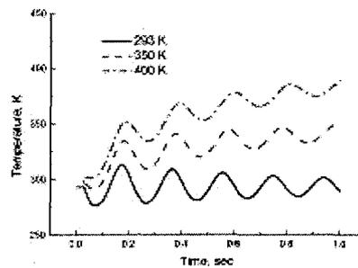
Fig. 14 The effect of ambient temperature on the average temperature inside bubble.
