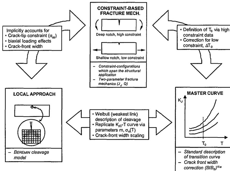
Figure 3: Schematic Illustration of interactions (integration) in the development of constraint-based fracture mechanics methodologies expected to result from the work of the VOCALIST group.
