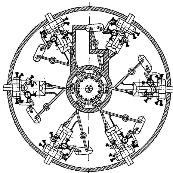
Fig. 1. General view of RBEC reactor
