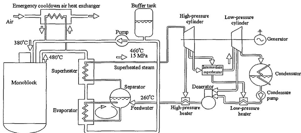
Fig. 3. Diagram of the RBEC intermediate and turbine circuits
