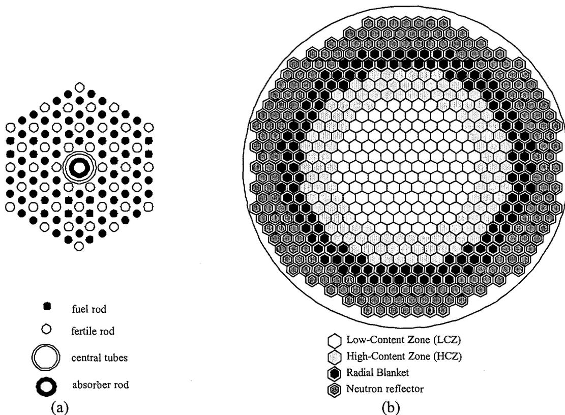
Fig. 2. RBEC core (a) and fuel assembly (b)
