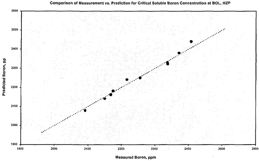
Figure 3. Comparison of the predicted and measured critical boron concentration at BOC, HZP for reload cores employing the low concentration gad design.
