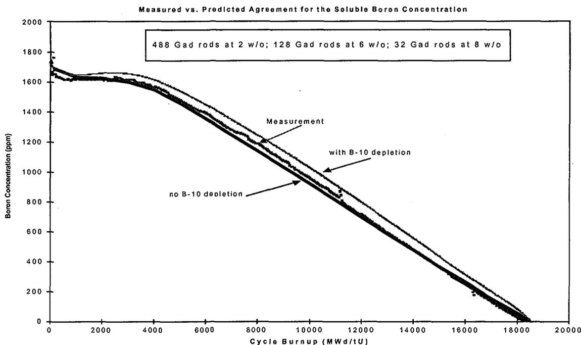
Figure 7. Typical (P-M) agreement for the critical boron concentration at HFP ARO during the depletion of the cycle for a reload core employing the low concentration gad design.
