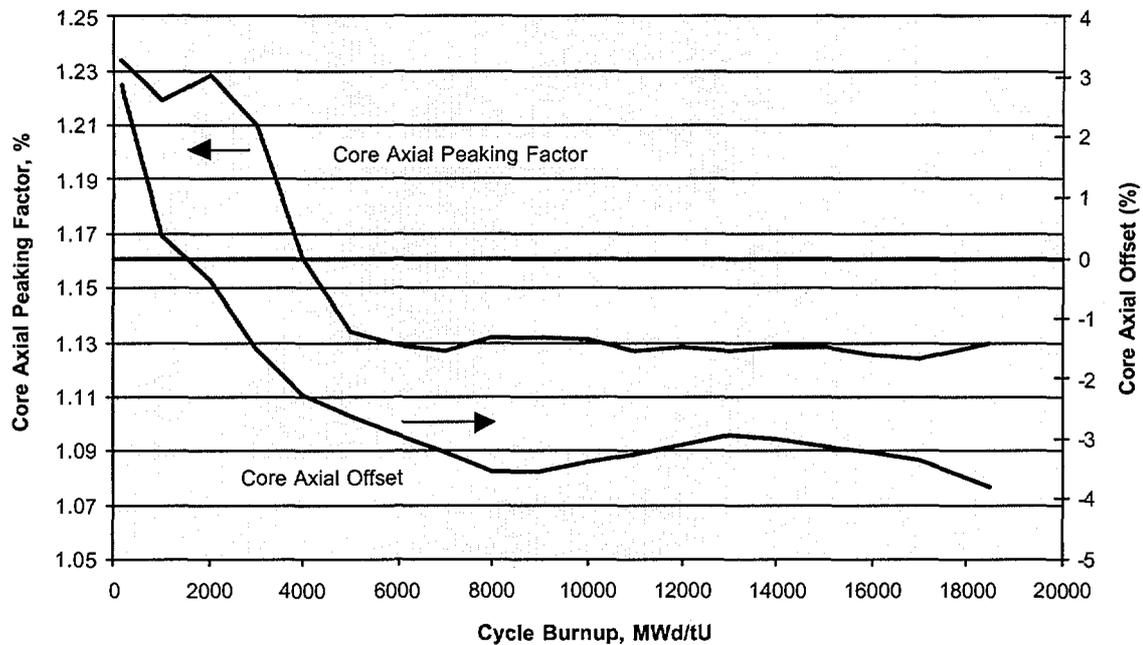
Figure 2. Typical behavior of the core axial peaking factor and axial offset for the low concentration gad design
