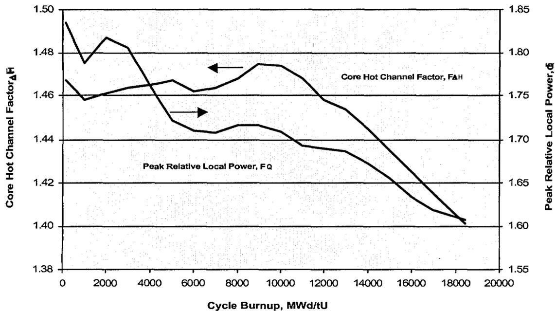
Figure 1. Typical behavior of the core maximum relative rod power,  $\bar{F}_{\Delta H}$ , and peak relative local power,  $\bar{F}_Q$ , for the low concentration gad design
