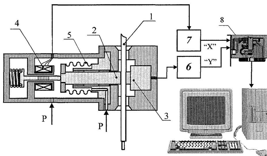
FIG.1. Schematic representation of the gap measurement facility: 1-fuel rod; 2-loader rod; 3-piezoelectric force transducer; 4-LVDT; 5-silphon; 6-charge amplifier; 7-normalizing amplifier; 8-analog/digital converter (ADC).
