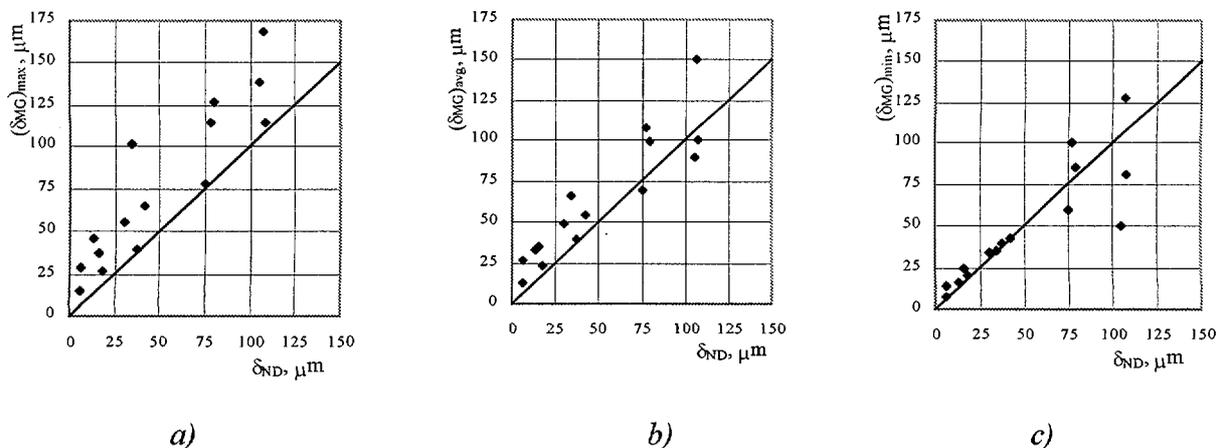
FIG. 6. Comparison of the diametrical gap values determined by the compression method ( $\delta_{ND}$ ) with the maximum (a), average (b) and minimum (c) gap values measured by metallography: — line of equal values ( $\delta_{ND} = \delta_{MG}$ ).
