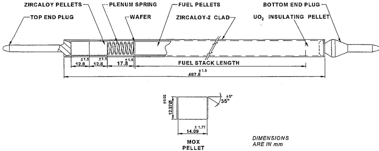
Fig. 1. A typical experimental mox fuel pin.
