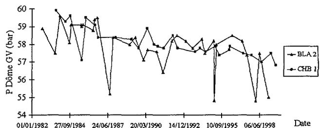
Figure 1 : Example of steam pressure drop at SG outlet of Chinon B1 CP2 unit and Blayais CP1 unit.
