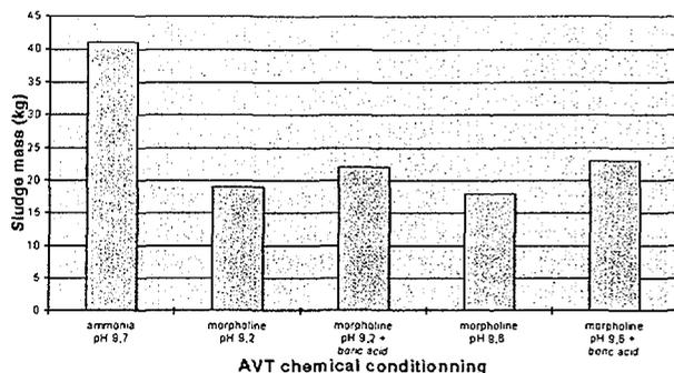
Figure 2 : comparison of sludge removed by lancing in some EDF PWRs units with various treatments.
