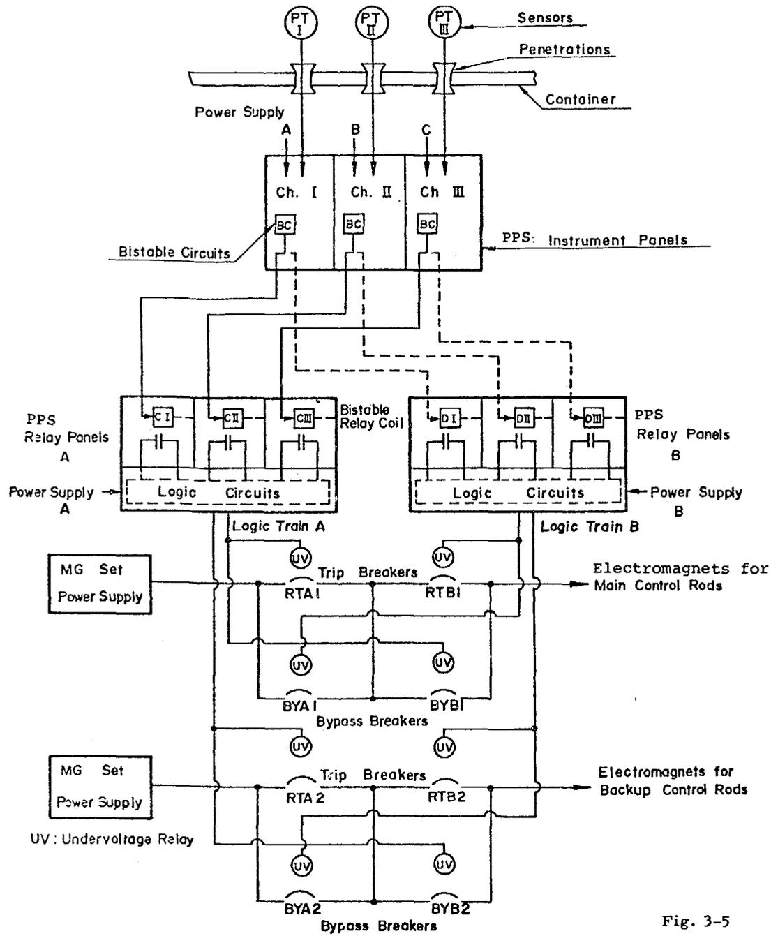
Fig. 3-5 Plant Protection System Instrumentation
