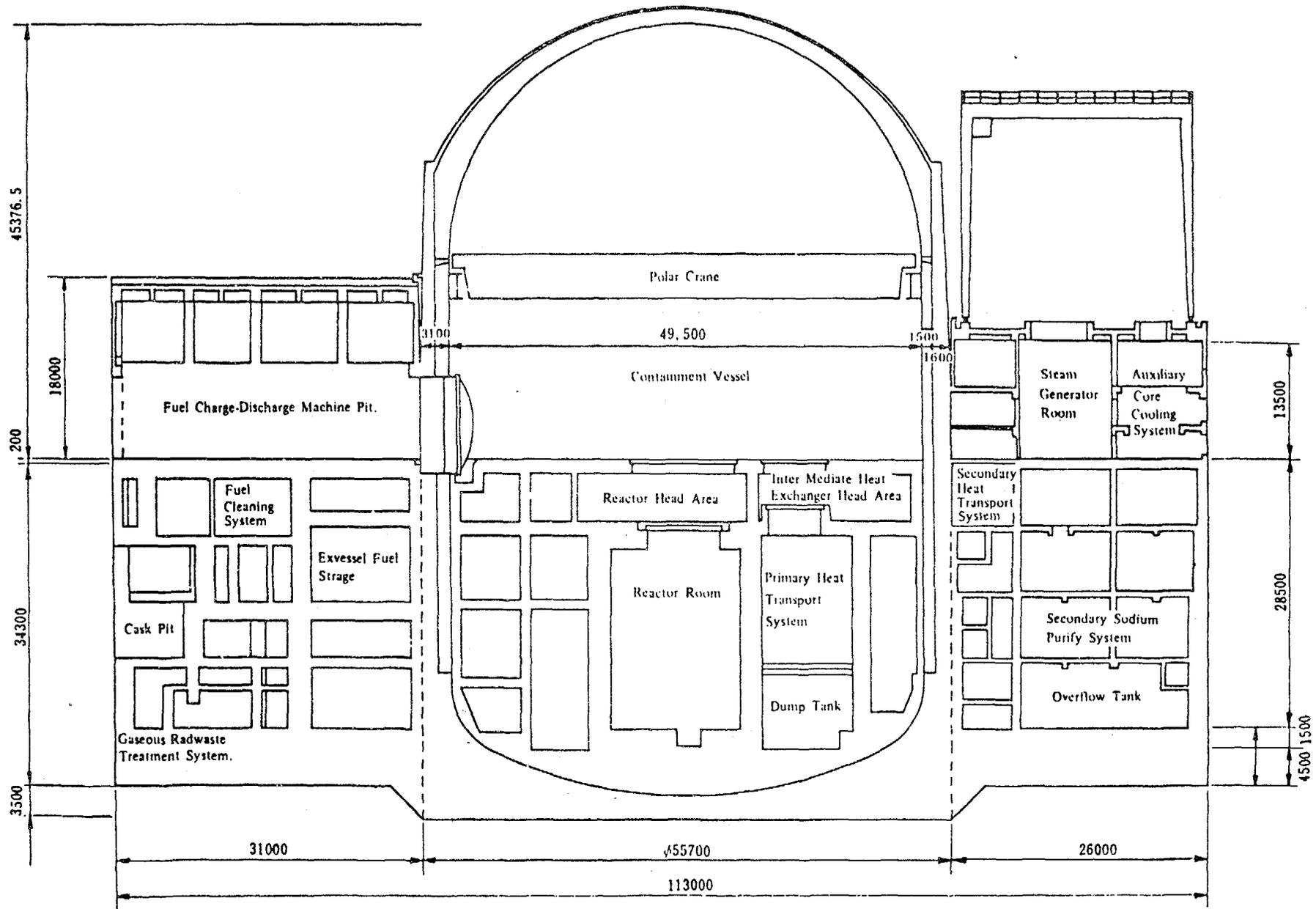
Fig. 3-7 Sectional Elevation of Reactor Building
