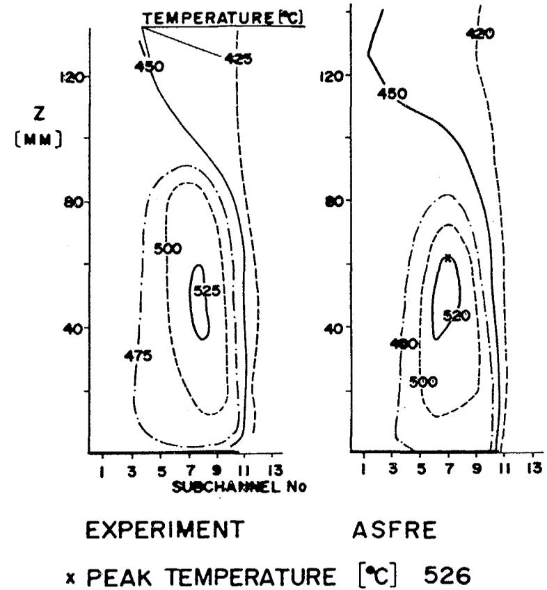
Fig. 11-1 Benchmark Calculation 49% Central Blockage Run No.1 Comparison of Temperature Distribution
