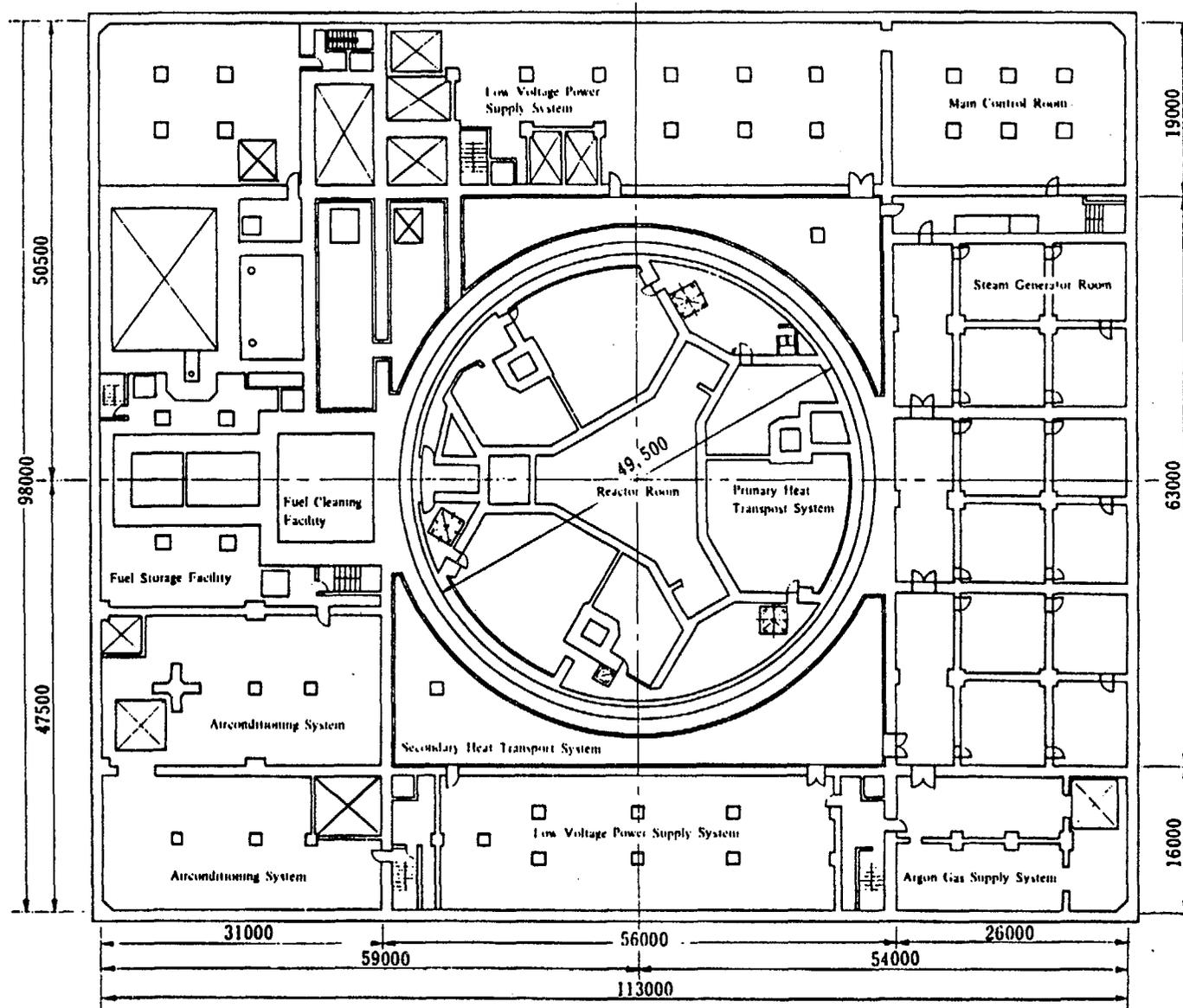
Fig. 3-8 Horizontal Cross Section Reactor Building
