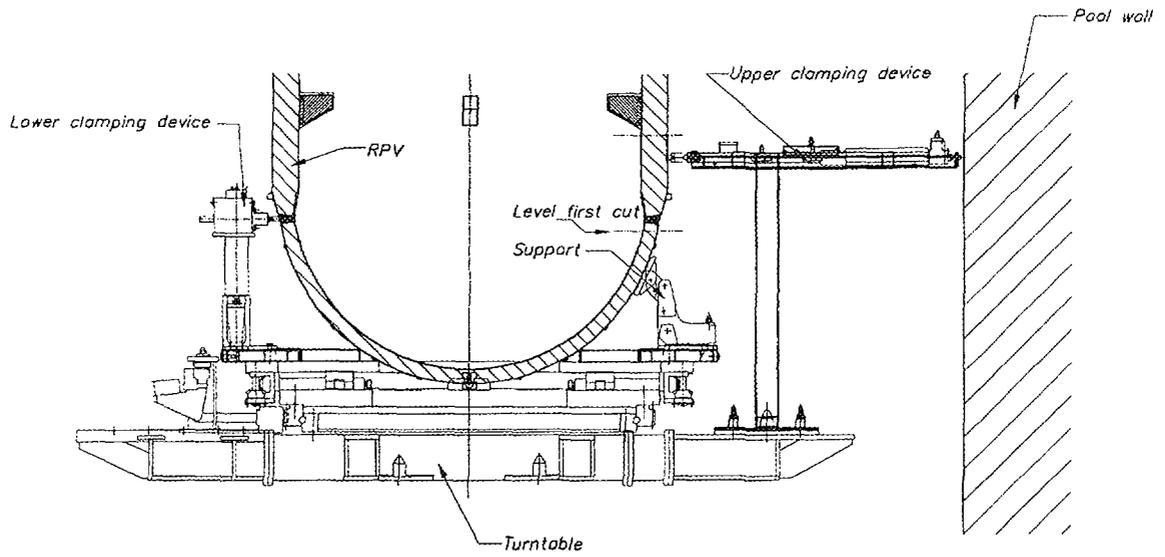
Figure 3. The spherical shape of the RPV bottom required additional clamping devices.
