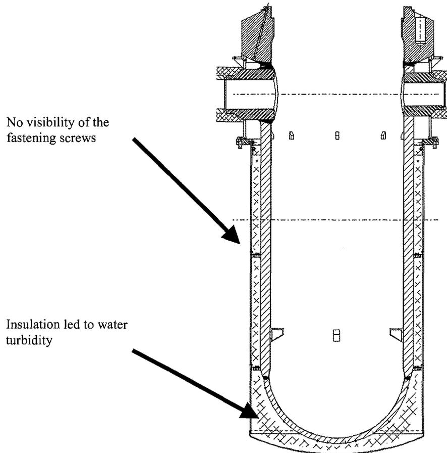
Figure 8. Second major problem: no visibility of the screw implied additional operation and the insulation led to pool turbidity.
