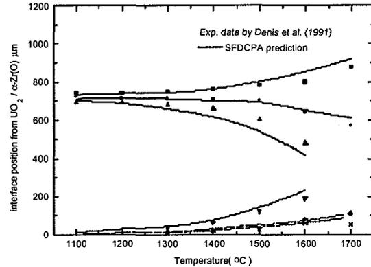
Fig.10 Various interface position for transient experiments at 10K/s and comparison with SFDCPA prediction.
