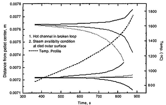
Fig. 11 Fuel pin condition in hot channel broken loop with steam availability at clad outer surface.
