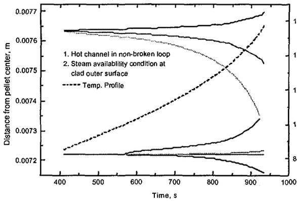
Fig. 13 Fuel pin condition in hot channel non-broken loop with steam availability at clad outer surface.
