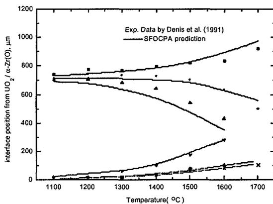
Fig.9 Various interface position for transient experiments at 5K/s and comparison with SFDCPA prediction.
