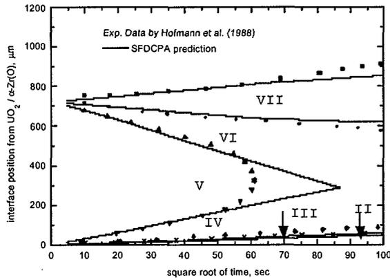
Fig.7 Various interface position for isothermal experiments at 1100°C and comparison with SFDCPA prediction.
