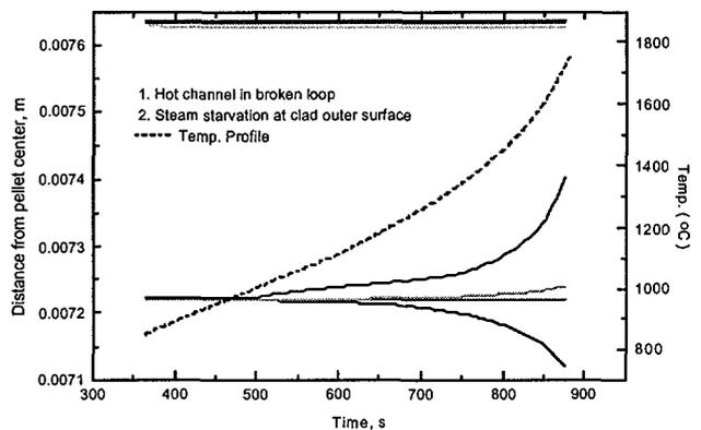
Fig. 12 Fuel pin condition in hot channel broken loop during steam starvation condition.
