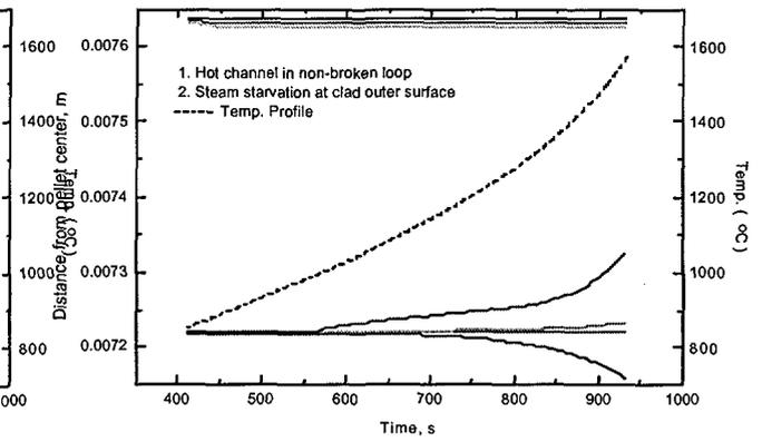
Fig.14 Fuel pin condition in hot channel non-broken loop during steam starvation condition.
