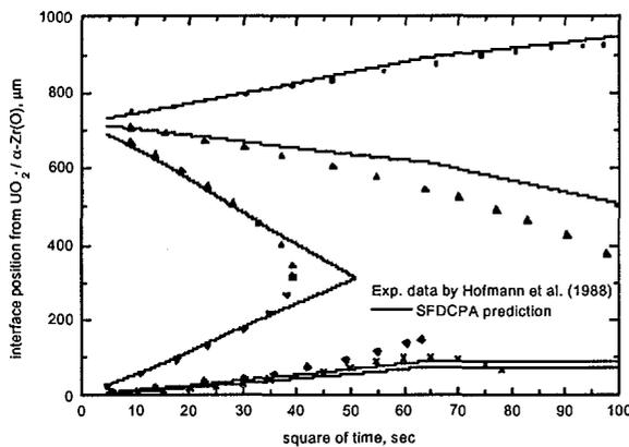
Fig.8 Various interface position for isothermal experiments at 1200°C and comparison with SFDCPA prediction.
