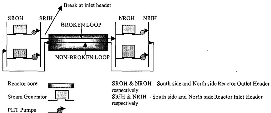
Fig.6 PWR System simulated by RELAP4 / MOD6
