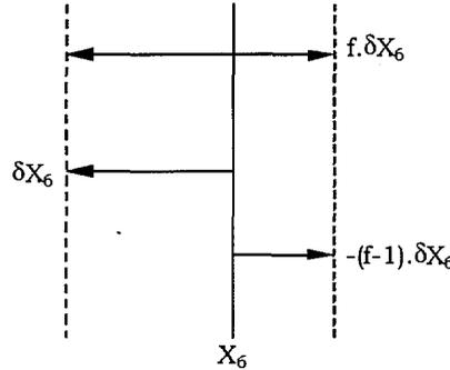
Fig.4 Change in layer thickness due to volumetric expansion
