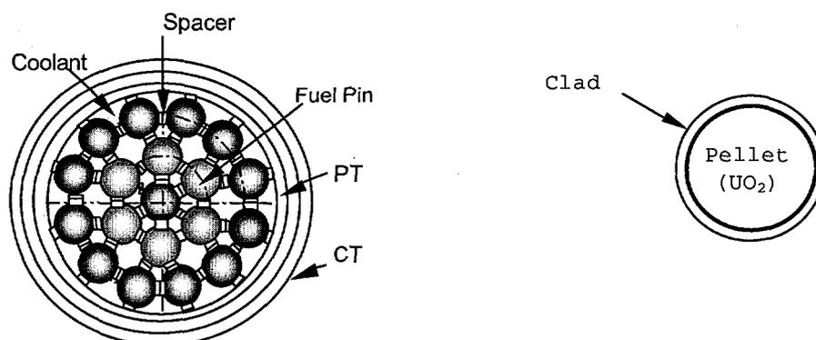
Fig.1 Reactor channel configuration
