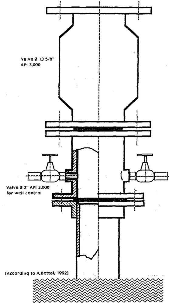
Fig.10.2. Example of production well head for wells of the shallow reservoir
