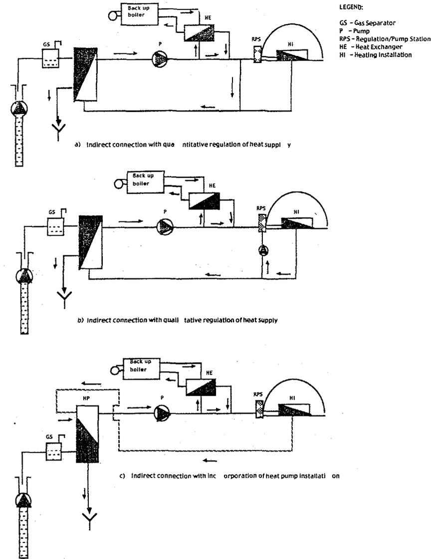
Fig. 5. Basic type of indirect connection to geothermal well(s)
