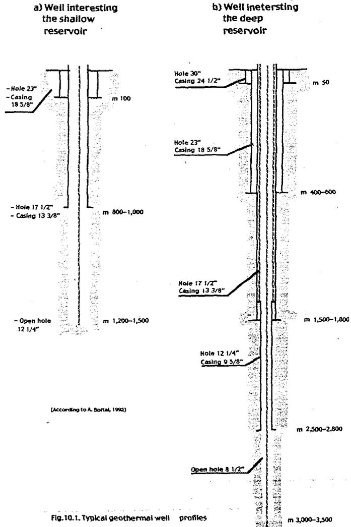
Fig.10.1. Typical geothermal well profiles
