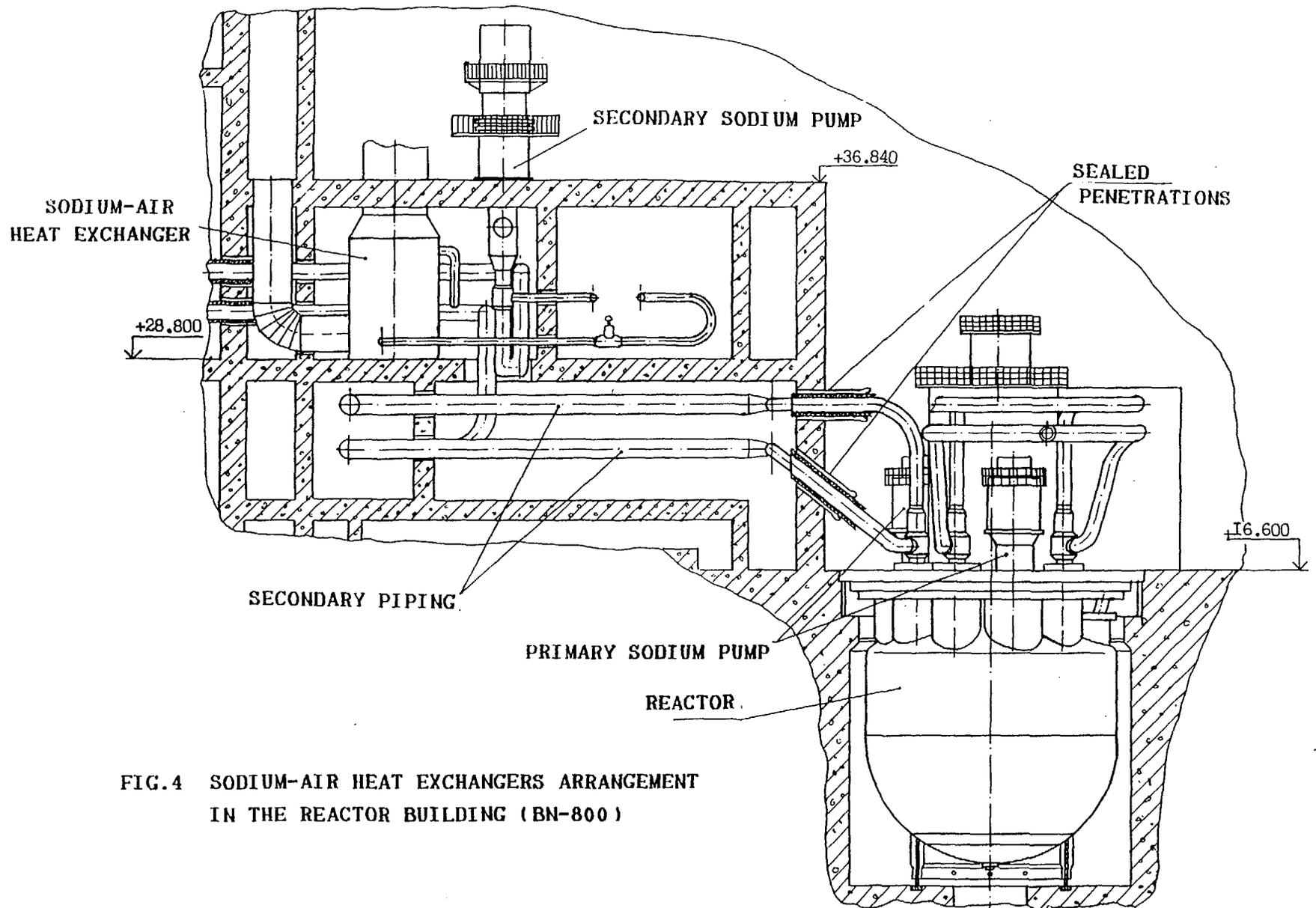
FIG. 4 SODIUM-AIR HEAT EXCHANGERS ARRANGEMENT
