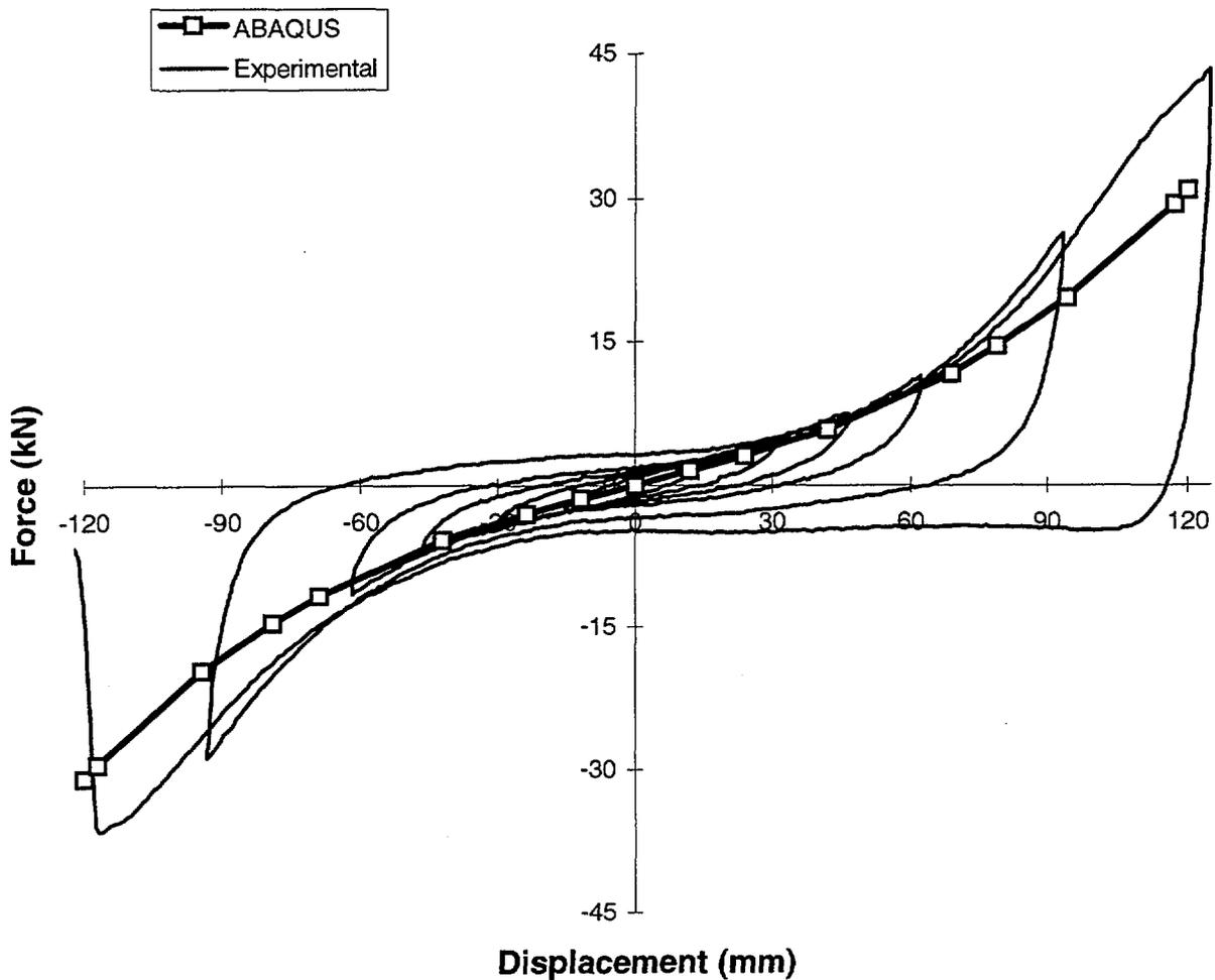
Figure 7-c. Experimental and numerical force-displacement values for a combined compression & 400% shear strain failure test on a bolted 'further optimized' HDRB (1:4 scale, diameter=125 mm, H=30 mm, S=12, G=0.4 MPa)
