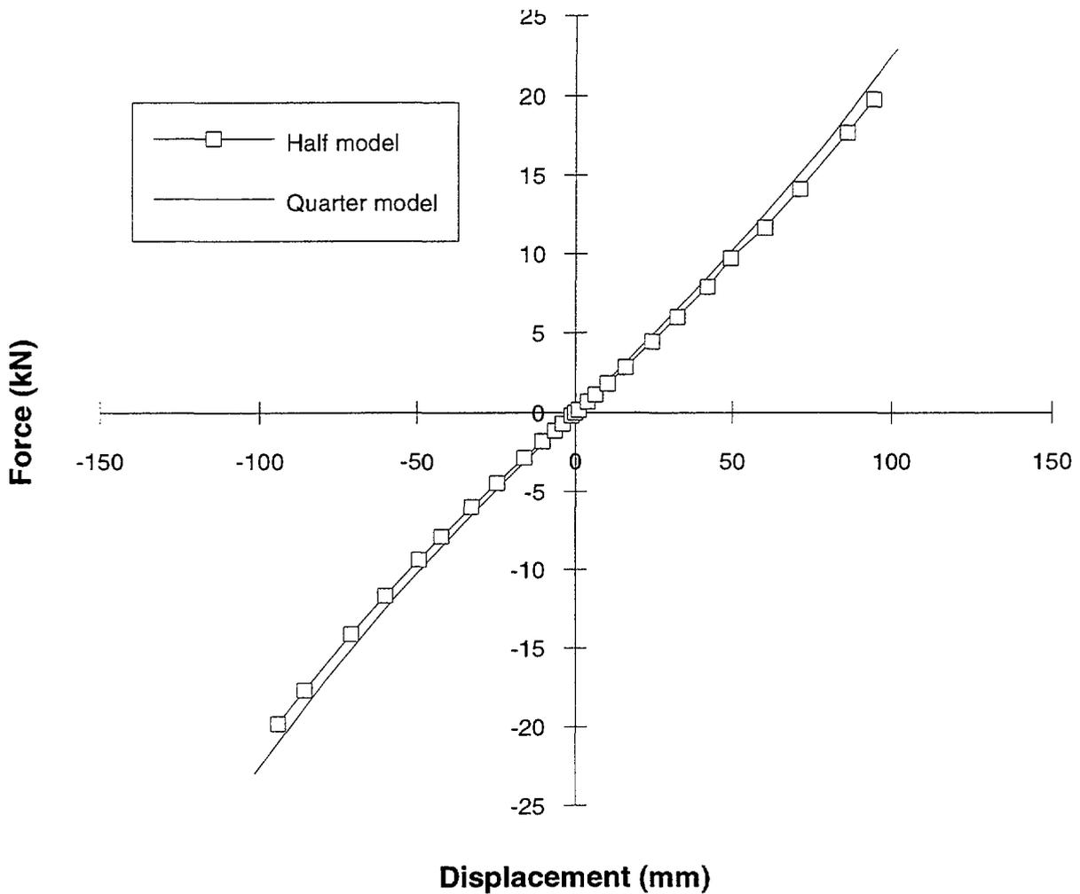
Figure 3-c. Comparison between the horizontal stiffnesses of HDRB in half scale using the FEMs of figures 3-a and 3-b
