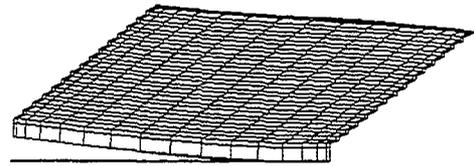
Figure 5-b. A quarter FEM of an optimized HDRB with recess attachment system at 200% shear strain
