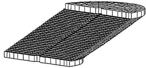
Figure 4-b. FEM of a bolted optimized HDRB at 300 % shear strain
