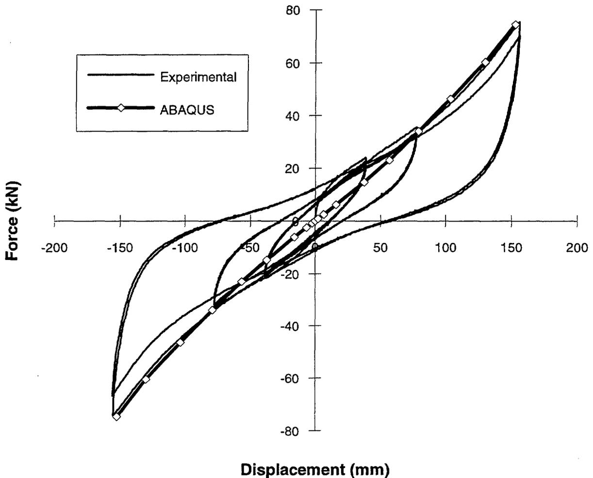
Figure 5-c. Experimental and numerical force-displacement values for a combined compression & 200% shear strain test on an optimized HDRB (1:2 scale, diameter=250 mm,  $H=75$  mm,  $S=24$ ,  $G=0.8$  MPa, recess attachment system)
