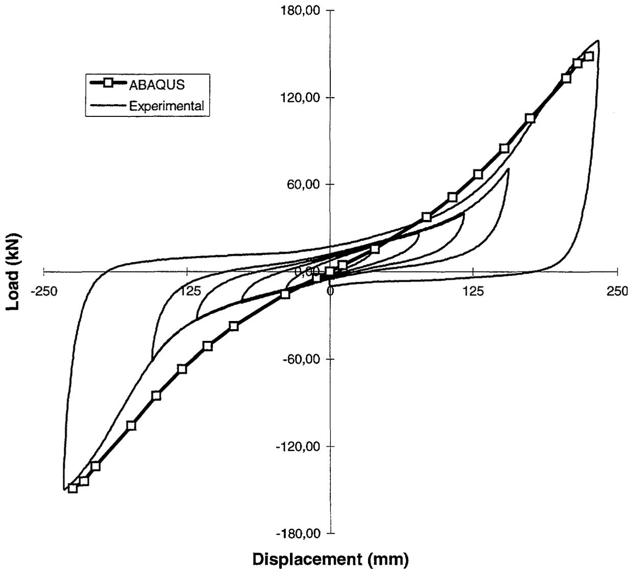
Figure 4-c. Experimental and numerical force-displacement values for a combined compression & 300% shear strain test on a bolted 'optimized' HDRB (1:2 scale, diameter=250 mm, H=75 mm, S=24, G=0.8 MPa)
