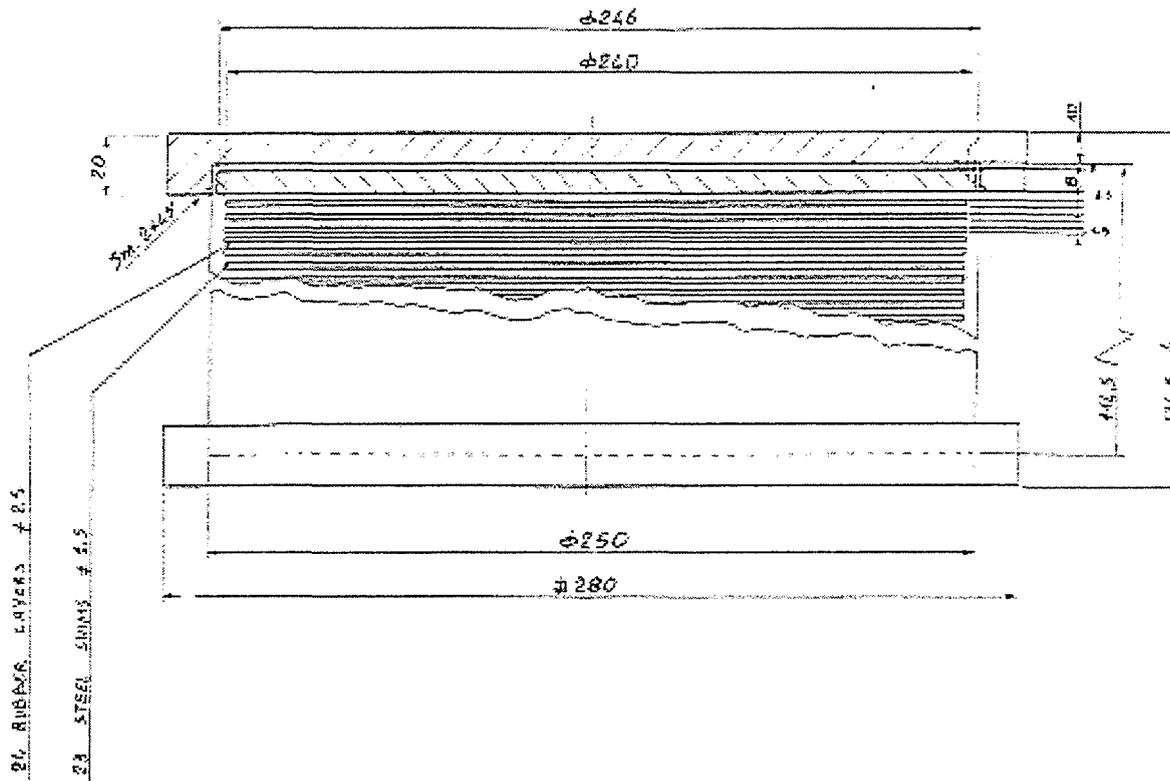
Figure 1. 'Further optimized' HDRB (250 mm diameter, 60 mm total rubber height, recess attachment system)
