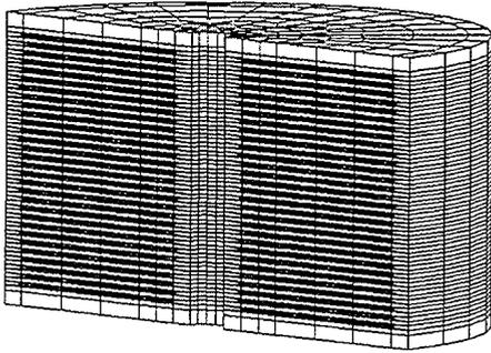
Figure 3-a. FEM of HDRB with symmetry about a vertical axial plane (YSYMM conditions) - Half model
