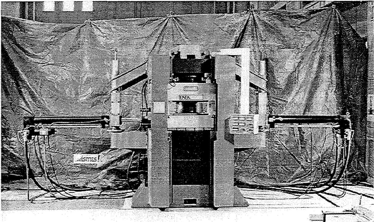
Figure 2. Optimized HDRB under testing on SISTEM machine.
