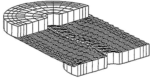
Figure 7-b. FEM of a bolted 'further optimized' HDRB at 400% shear strain
