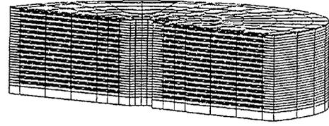
Figure 3-b. FEM of HDRB with symmetry about a vertical axial plane and hemi-symmetry - A quarter model
