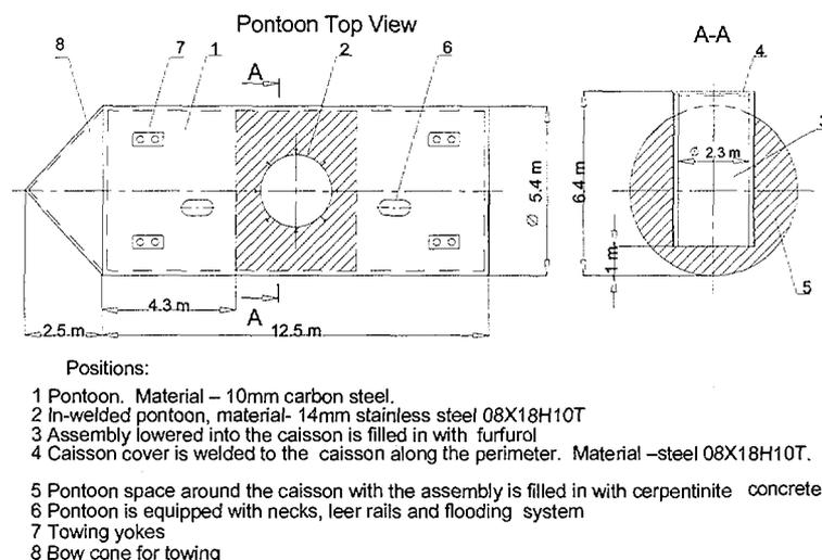
Fig. 1. Scheme of pontoon assembly 02.
