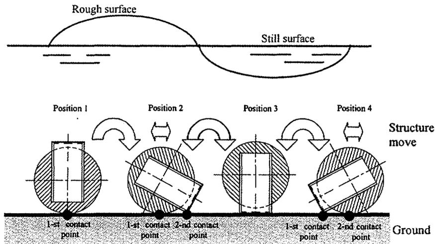
Fig. 2. Dynamics of pontoon motion at 10 to 20m depth, under the action of loads from currents and seaways.
