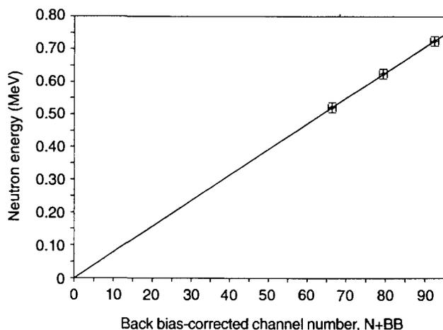
Figure 5. Data from measurements with monoenergetic neutrons and SP2-10 detector: symbols, from measurements; line, fit to measured data. See text and Equation 10 for explanation of (N+BB).
