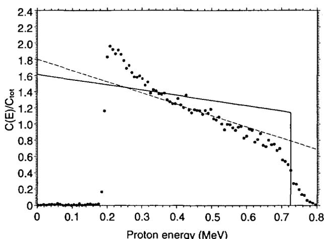
Figure 3. Response function for 725 keV neutrons in SP2-10 detector (10 atm. H<sub>2</sub>): solid line, calculated with Snidow algorithm; symbols, measured data; dashed line, fit to measured data between 400 and 500 keV.
