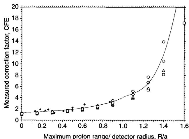
Figure 4. Correction factors as a function of 'maximum proton range/detector radius': filled symbols, from measurements in present work; open symbols, averages of data published in open literature; line, fit.
