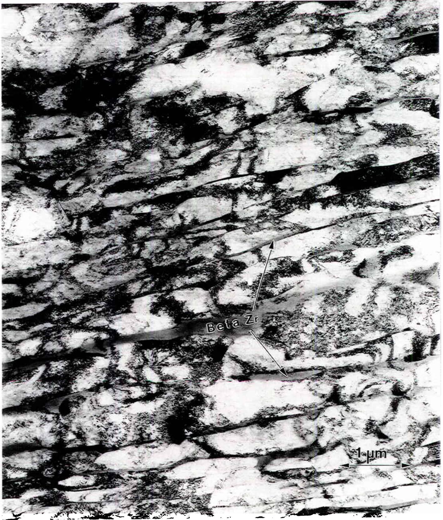
Figure 1. Typical pressure-tube microstructure, looking at the longitudinal/transverse plane, showing the predominant  $\alpha$ -Zr flattened grain structure surrounded by smaller amounts of  $\beta$ -Zr (gray areas).
