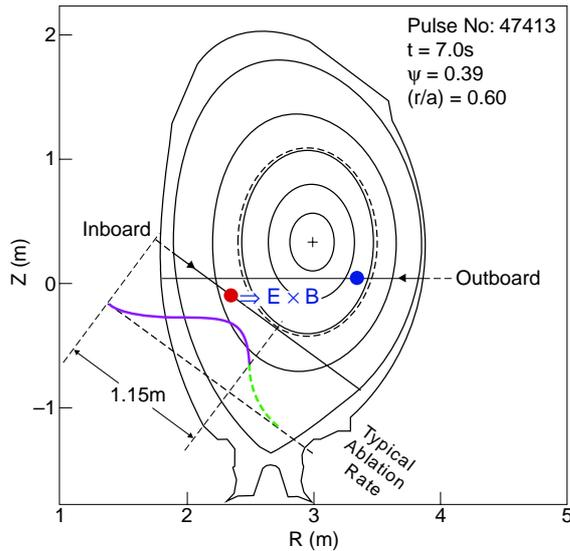
FIG. 1. Injection geometries of the JET centrifuge pellet injector.
