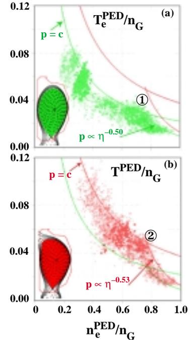
FIG. 4. Effect of triangularity  $\delta$  on H-mode pedestal density and temperature. At low  $\delta$  (a) the edge ballooning limit (green curve) is lower than at high  $\delta$  (b) (red curve). As the pedestal density is increased by gas puffing the pedestal pressure decreases as the square root of resistivity  $\eta$  starting at the same density (a-1, b-2).
