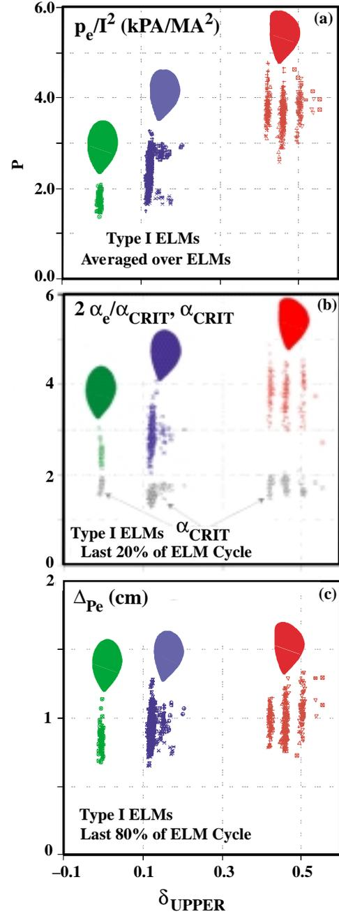
FIG. 3. Effect of upper triangularity  $\delta$  on the H-mode pedestal at moderate density. (a) Electron pressure at the top of the H-mode transport barrier showing a strong increase with  $\delta$ , (b) edge pressure gradient normalized to ballooning mode limit and value of  $\alpha_{\text{crit}}$ , (c) width of the steep edge electron pressure gradient region,  $\Delta_{pe}$ .
