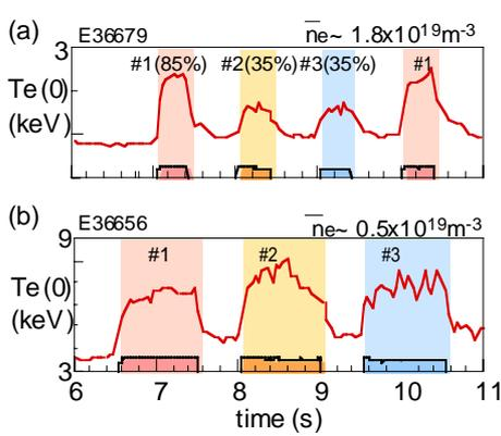
Fig.1 Multi-pulse injections of different power fraction of O-mode component ; (#1:85%, #2:35%, #3:35%). (a)  $\bar{n}_e \sim 1.8 \times 10^{19} \text{m}^{-3}$ , (b)  $\bar{n}_e \sim 0.5 \times 10^{19} \text{m}^{-3}$ .
