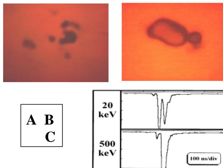
*FIG.1. Ion beam images obtained from many PF discharges (A) and from a single PF discharge (B) in the presence of hot spots emitting REBs (C).*
