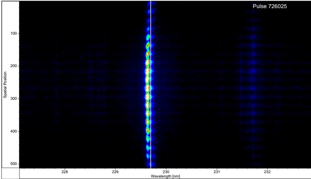
FIG. 4 - C III line (229.7 nm) emission at 30  $\mu$ sec as viewed oblique to the plasma column using the iCCD imaging spectrometer. The spectra show Doppler shifts towards blue of the central plasma indicating an axial flow velocity of  $9.6 \times 10^4$  m/s and no Doppler shift of the outer plasma. The solid line is positioned at 229.7 nm for reference.
