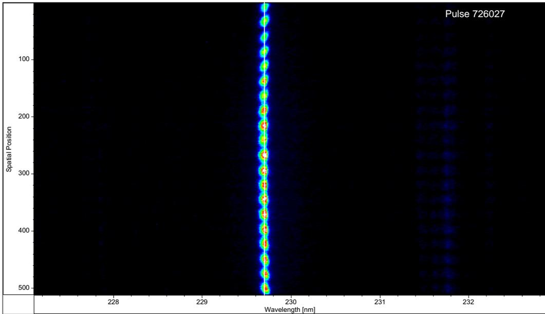
FIG. 5 - C III line (229.7 nm) emission at 38  $\mu$ sec as viewed oblique to the plasma column using the iCCD imaging spectrometer. The spectra show significantly reduced Doppler shifts and broader lines. The solid line is positioned at 229.7 nm for reference.
