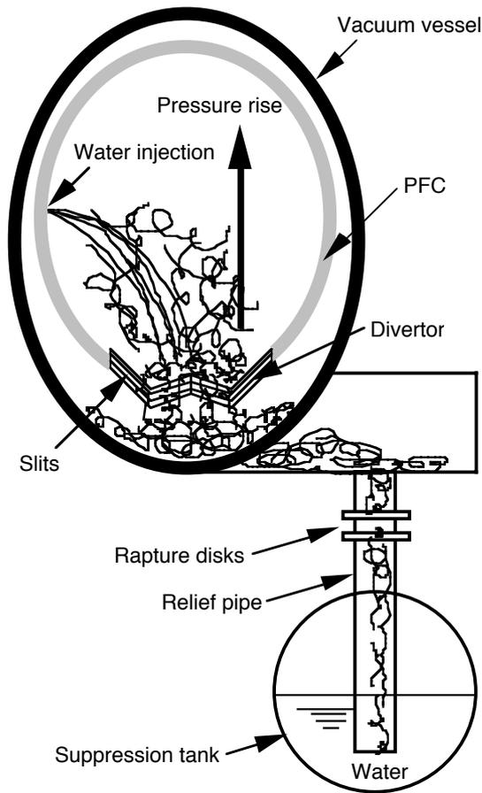
FIG. 1 ITER pressure suppression system.
