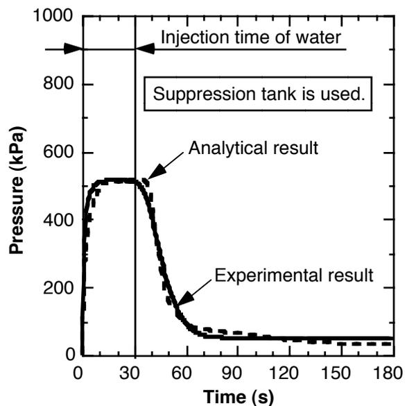
FIG. 6 Pressure transients in the PC at Case 3.
