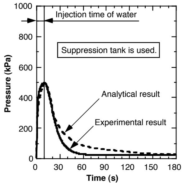
FIG. 5 Pressure transients in the PC at Case 2.
