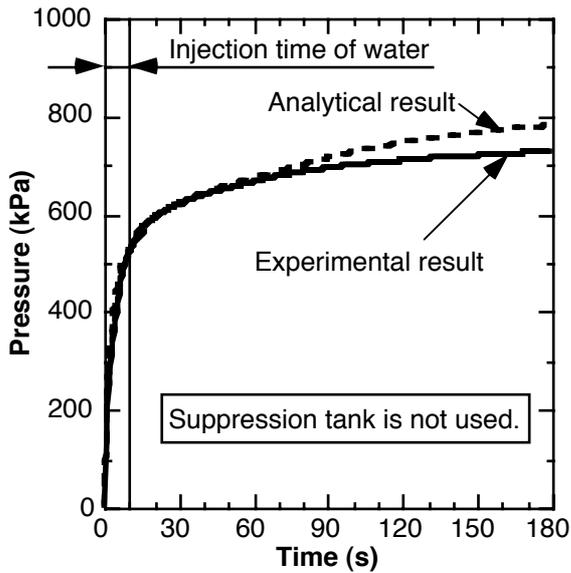
FIG. 4 Pressure transients in the PC at Case 1.
