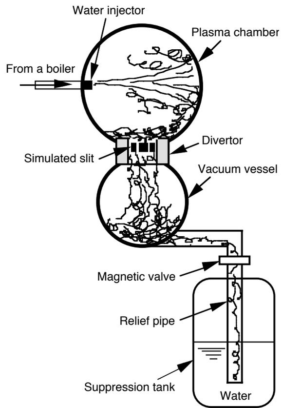
FIG. 2 Outline of an integrated ICE test facility.
