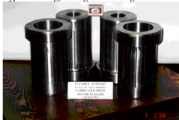
FIG. 6 RFHT flexible cartridge prototypes
