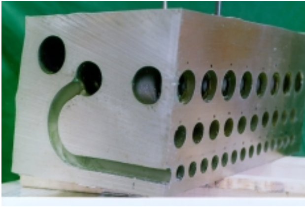
FIG. 3 EUHT powder HIP module destructive examin. FIG. 4 JAHT blanket prototype completed
