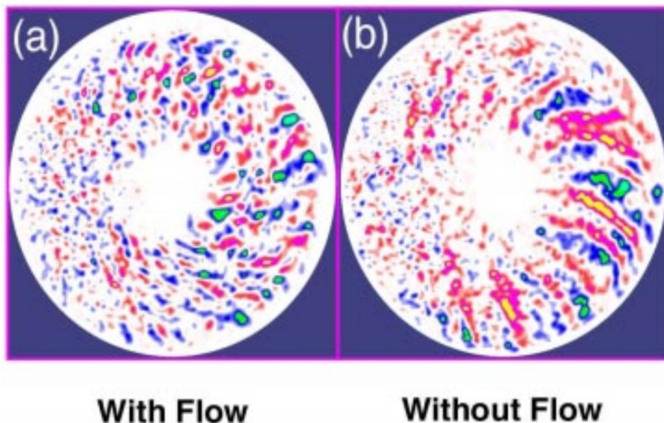
Figure 3: *Three-dimensional Particle Simulations of Zonal Flow Effects*
