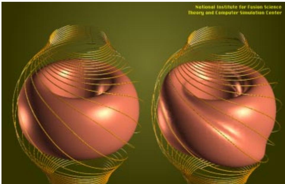
Figure 4: *MHD Simulation of Internal Reconnection Event in a Spherical Torus*
