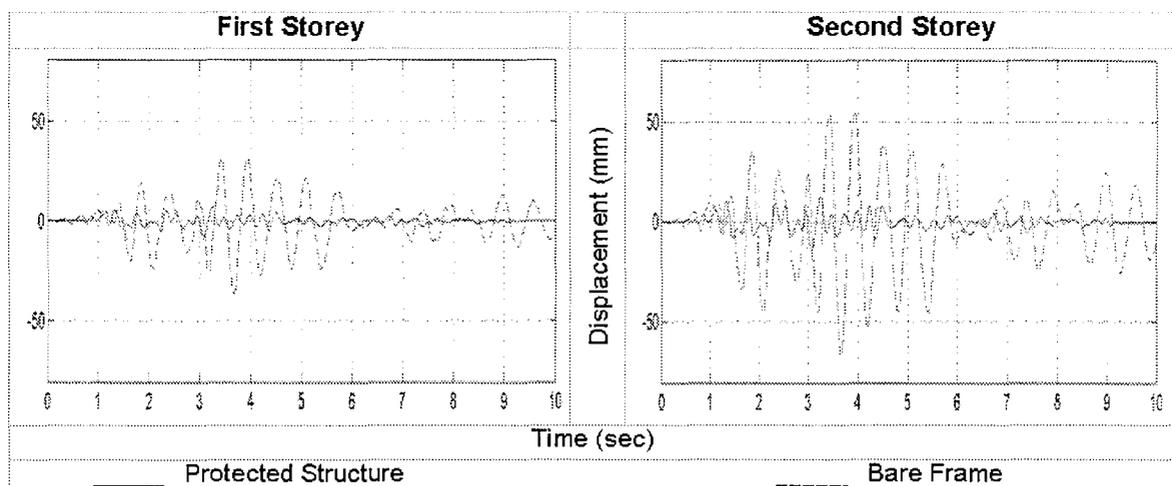
Figure 19: Displacement comparison between PsD tests of the protected structure and bare frame.
