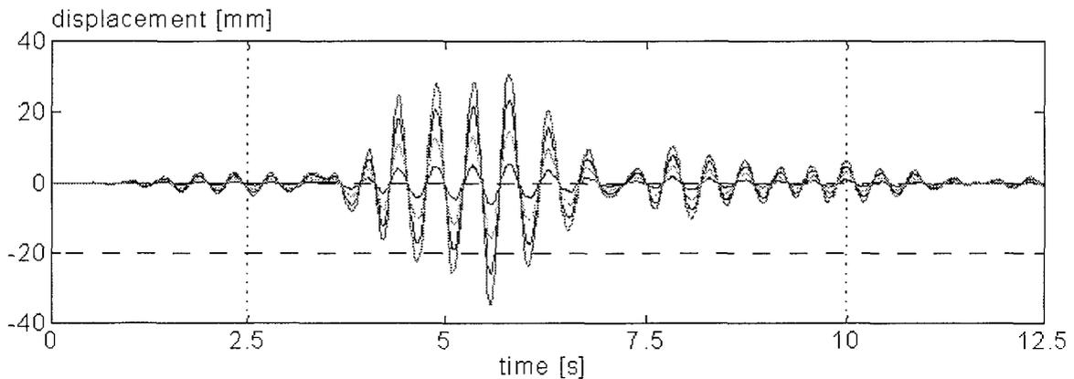
Figure 8: Non-isolated structure seismic PsD test: floor 1,2,3,4 displacements.
