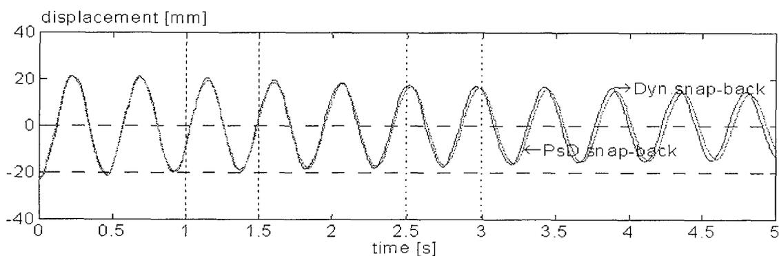
Figure 4: Non –isolated structure: Comparison of displacement time history at 4<sup>th</sup> floor for the dynamic and PsD snap-back tests.
