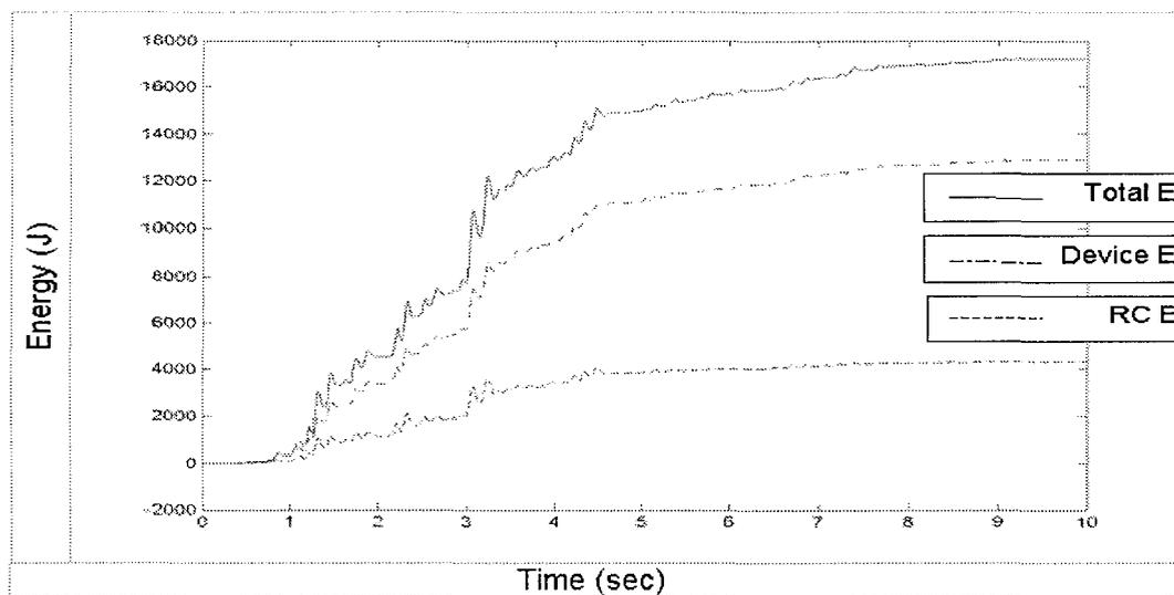
Figure 21: Energy absorbed during the PsD test of the protected structure.
