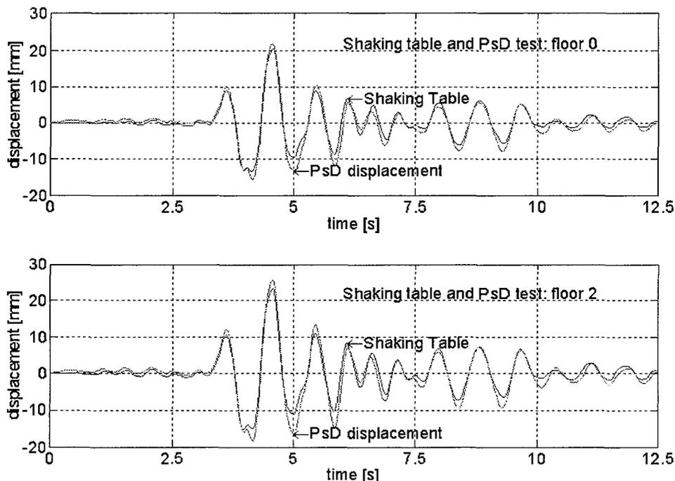
Figure 13: Isolated structure.-6dB Tolmezzo Earthquake: floor 0 and 2 displacements Shaking table and PsD tests comparison.
