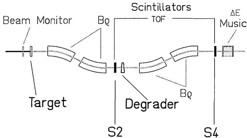
Figure 1: Schematic drawing of the fragment separator FRS and its detector equipment. The beam monitor measures the incident ions number. Scintillators provide magnetic rigidity and time of flight of the fragment. MUSIC chambers give nuclear charge.
