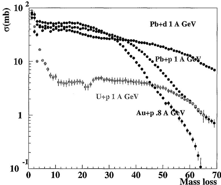
Figure 2: Production cross section as a function of the mass loss with respect to the projectile, measured with inverse kinematics method for projectile fragmentation in systems Au+p at 800 A MeV, Pb+p at 1 A GeV, Pb+d at 1 A GeV, U+p at 1 A GeV. Fission is not included.
