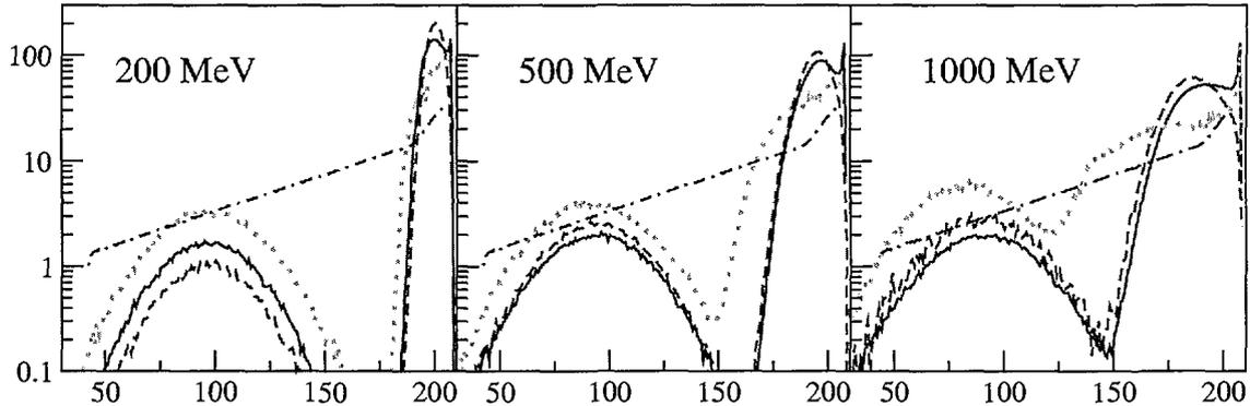
Figure 5: Residues production cross section predictions as a fonction of the mass for projectile energies 200 MeV, 500 MeV and 1 GeV (left to right) in the  $H+Pb$  reaction. Green discontinuous line, violet continuous line, orange dotted line the red dotted-dashed line represent respectively calculations by INCL+ABLA, Isabel+ABLA, Bertini+Dressner and EPAX.
