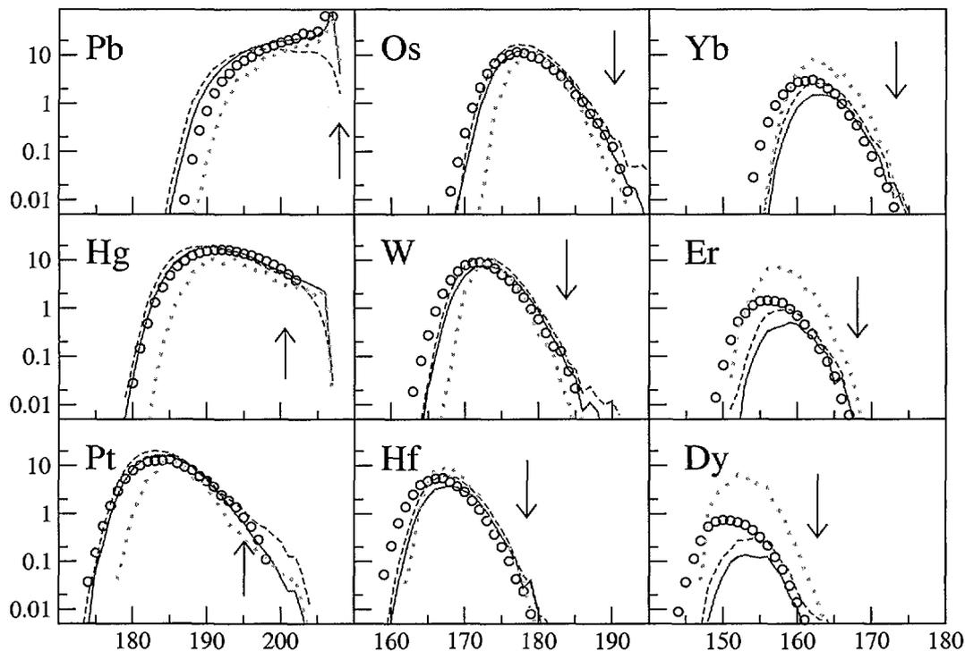
Figure 4: Fragmentation residues production cross section as a function of the mass for even  $Z$  values between 66 and 82 in the  $H+Pb$  at 1 GeV reaction. Experimental data are plotted as circles. Lines represents codes calculations: Isabel+ABLA (continuous line), INCL+ABLA (discontinuous line), LAHET (crosses). Vertical arrows indicate mean mass of stable isotopes.
