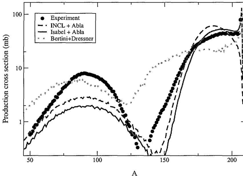
Figure 3: *Production cross section as a fonction of the mass of the residue in the H+Pb at 1 GeV reaction, from experimental data and from Monte-Carlo simulation codes.*
