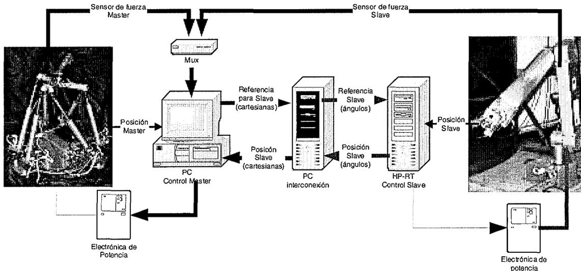
Figure 7. Interconnection scheme plan of the different components of Maliba
