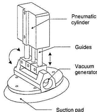
Figure 15 Vacuum system and pads positioning/ orientating system.
