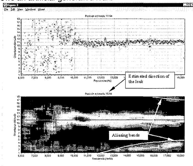
Figure 5. Location window. This window displays a system with a leak in the direction 11.
