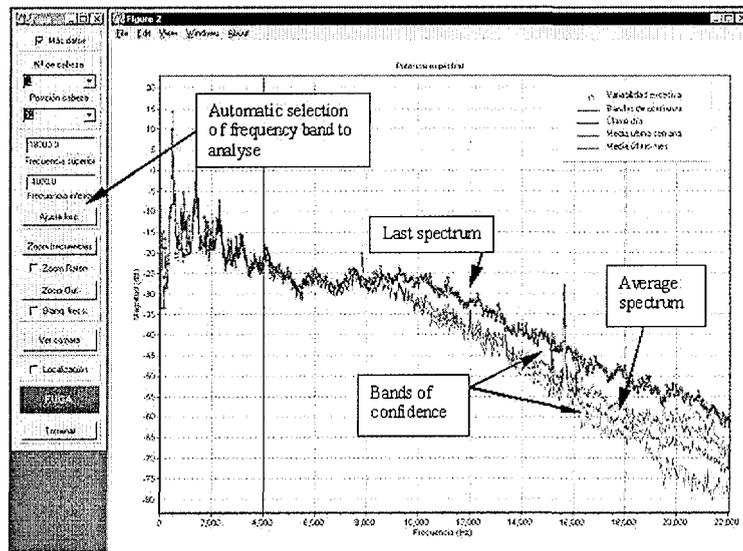
Figure 4. Leak detection window
