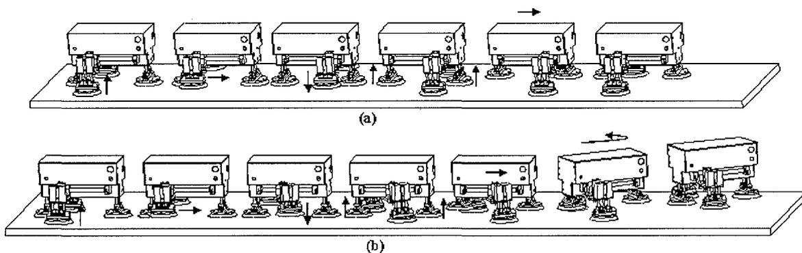
Figure 11 Steps to obtain forward (a) and rotation (b) motion.
