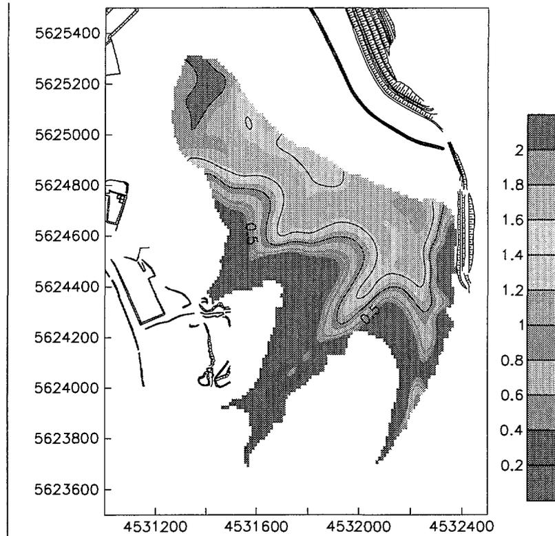
FIG. 8. Tailings Pond Helmsdorf: Spatial distribution of settlement portions under a cover load of 100 kPa in the fine tailings zone as derived from non-linear finite strain consolidation modeling.
