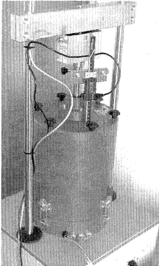
**in the foreground:** electromechanically driven automatic press with oedometer cell (red tube)
