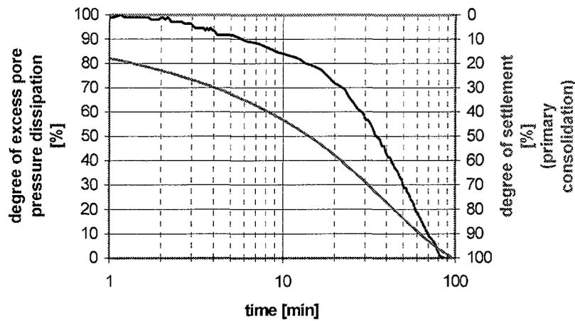
FIG. 5. Diagram: Example of measured time-settlement data on fine uranium mill tailings (WISMUT; Dep. of Eng.; geotechnical lab).
