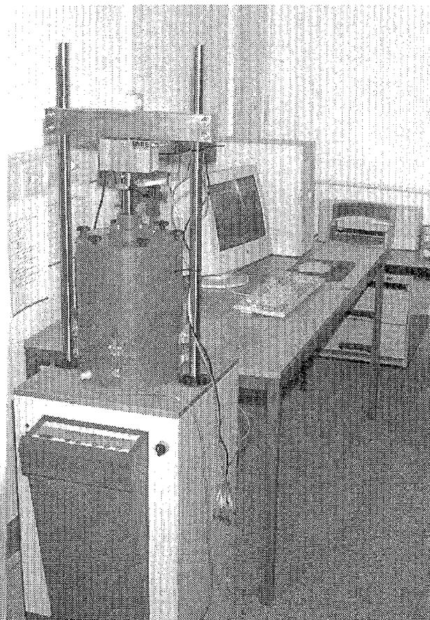
oedometer cell (internal diameter: 200 mm, max. samples height: 190 mm) measured test parameters:
