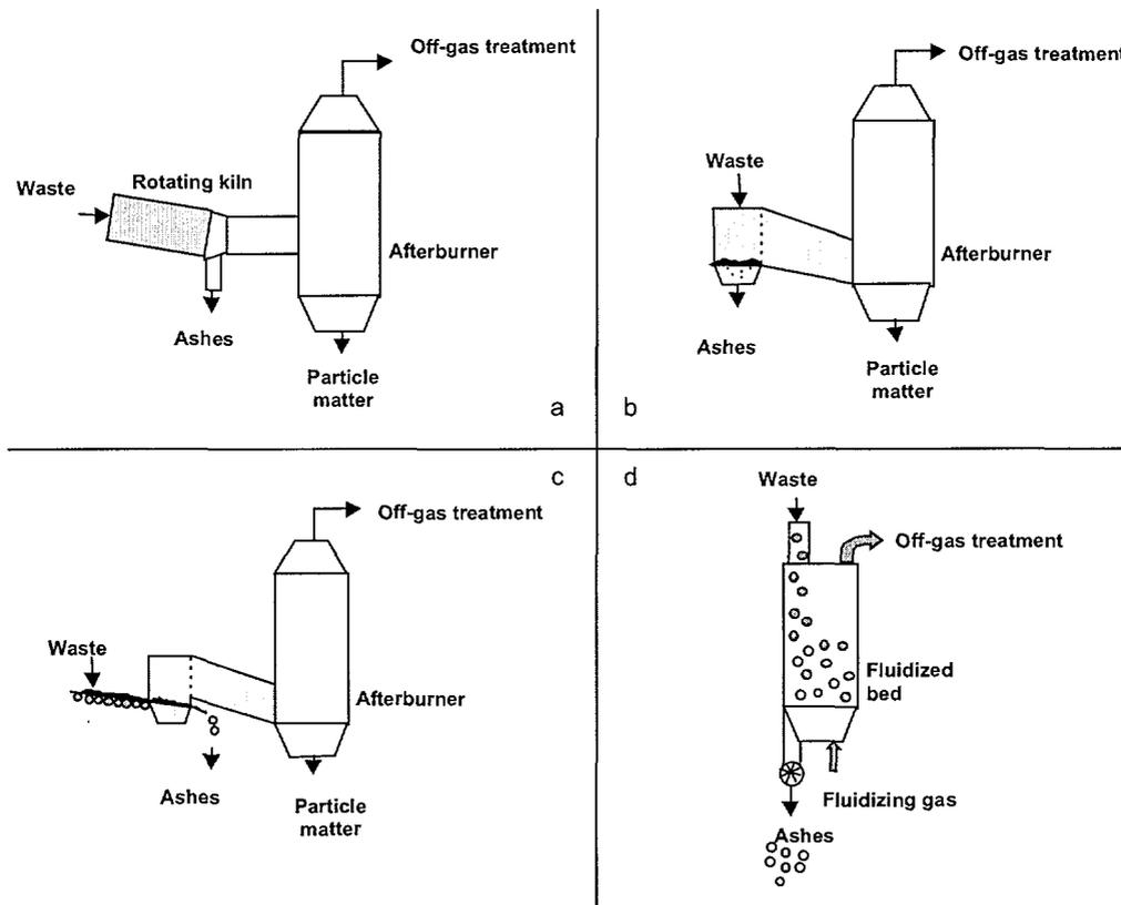
Figure 1. Various technologies suitable for high-rate waste incineration
