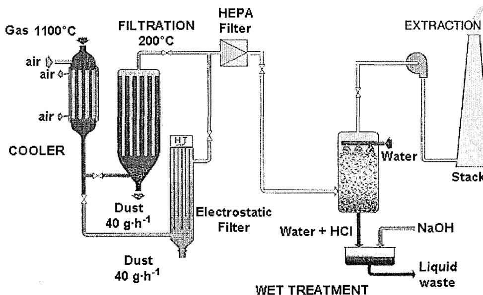
Figure 3. IRIS process off-gas treatment
