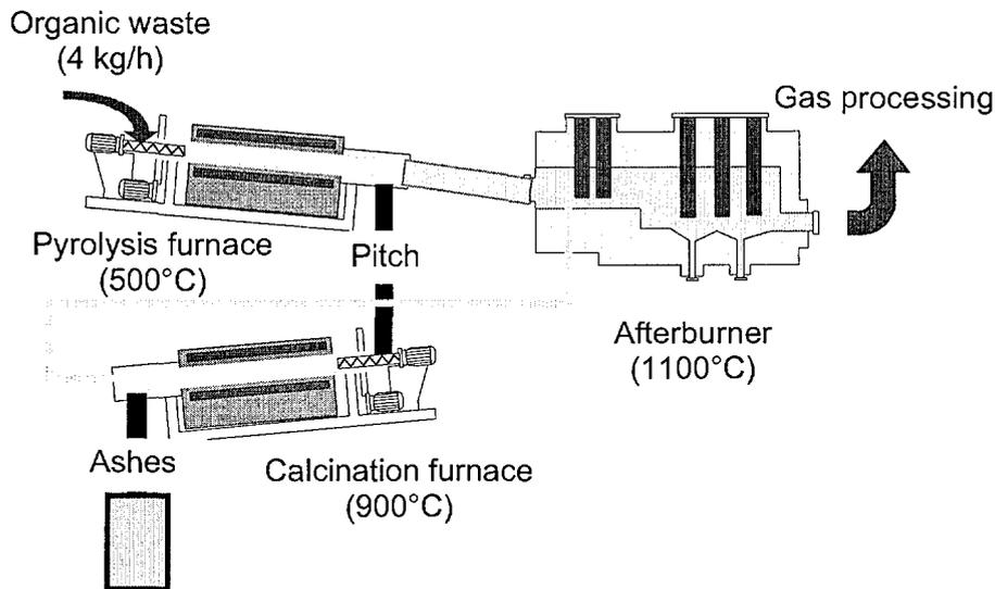
Figure 2. IRIS heat treatment cycle
