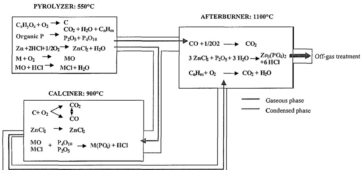
Figure 4. Overall material degradation schematic for the IRIS process
