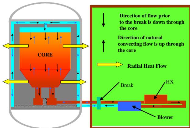
**Fig. 1 Schematic of pebble bed reactor and vault**
