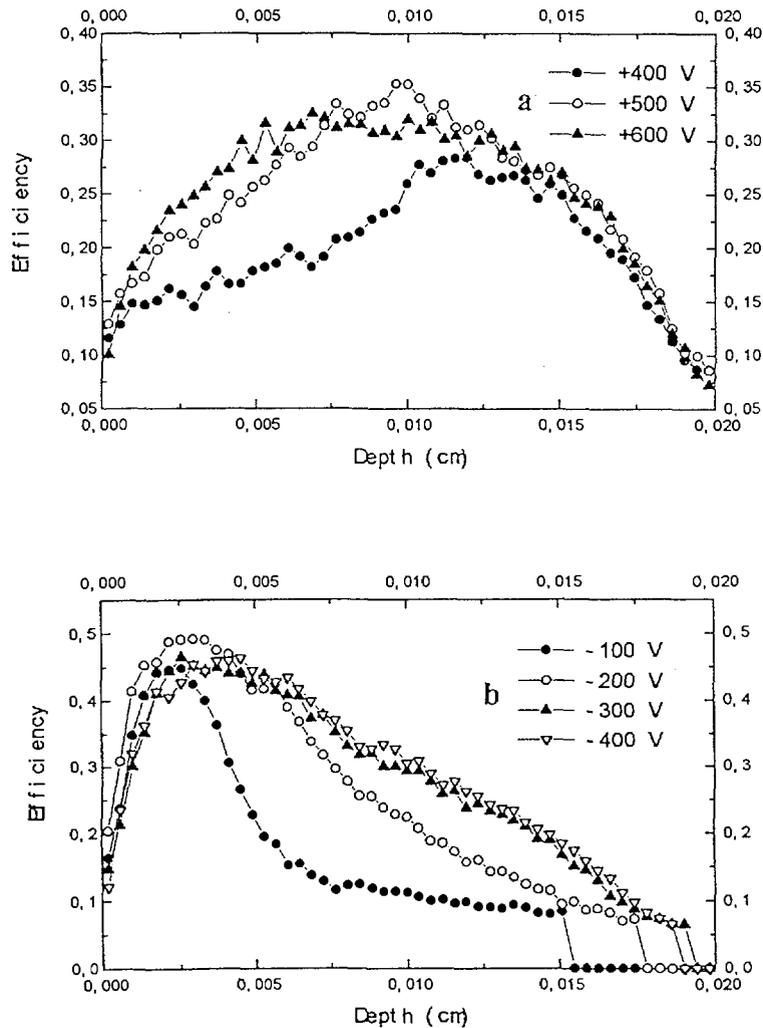
Fig. 7. Charge collection efficiency profile along the CVD diamond growth direction for positive bias (a) and negative bias (b). The growth side (biased) is on the left of the diagram.
