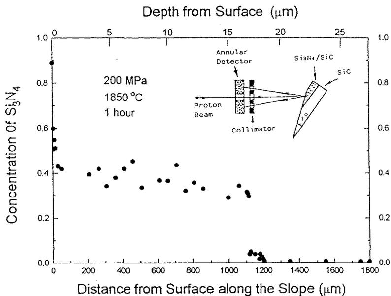
Fig. 2. Depth distribution of  $Si_3N_4$  molecular concentration in a layer of  $Si_3N_4/SiC$  composite ceramic on the silicon carbide surface. A diagram of the experimental setup is also displayed in the figure.
