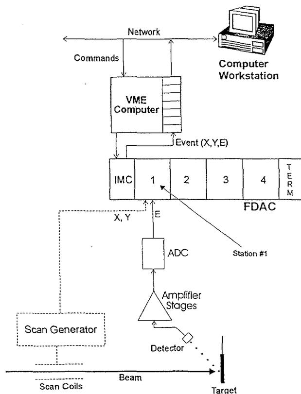
Fig.1. Schematic diagram of the general operation of the new multi-detector and multi-parameter data system hardware with a single detector providing input as a station example.
