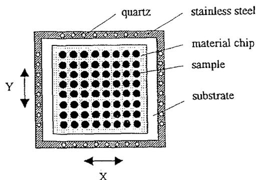
Fig. 8. Schematic of material chip holder for RBS and PEB analysis. The double arrow represent that the holder is able to move along X and Y directions to make the sample aligned with the analysing beam.
