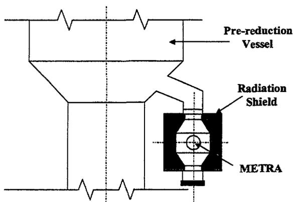
Figure 2. Schematic diagram of the NIS gauge METRA installed on a plant in Western Australia.
