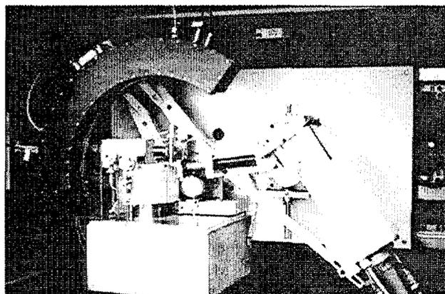
Figure 3. The upper cabinet of the on-line XRD instrument showing the position sensitive detector, continuous feed sample presenter and X-ray source.
