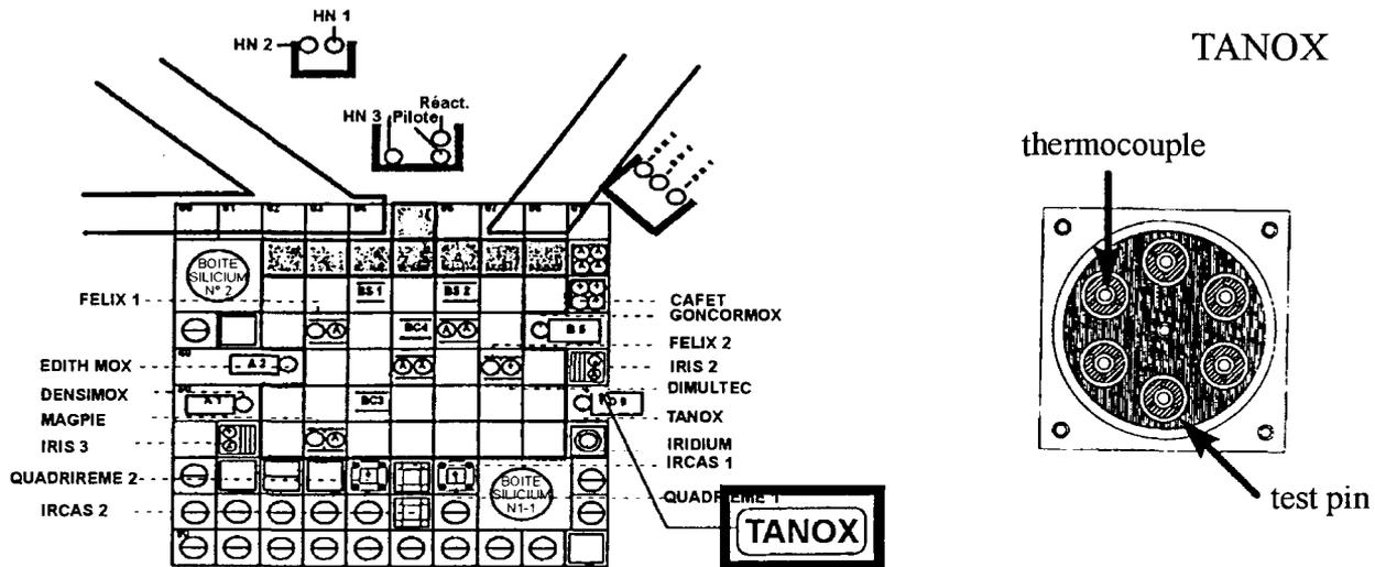
Fig. 2. TANOX device and in SILOE reactor location
