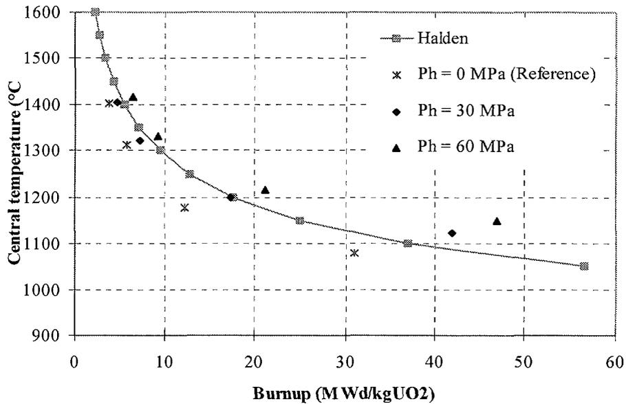
FIG. 1: The effect of the hydrostatic pressure on the central temperature for 1% average fission gas release versus burnup during irradiation at constant linear heat rate.
