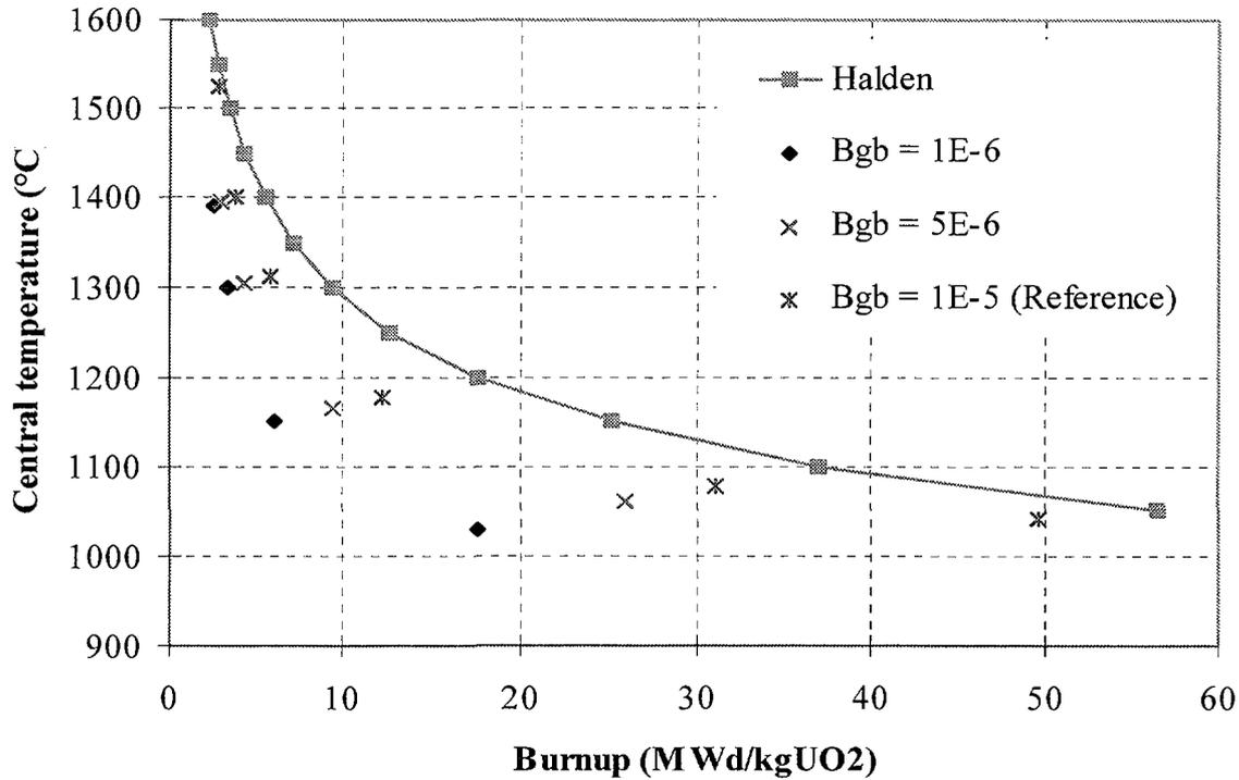
FIG. 5: The effect of resolution rate constant at the grain boundary for 20 kW/m ( $B_{gb}^{ref}$ ) on the central temperature for 1% average fission gas release versus burnup during irradiation at constant linear heat rate.
