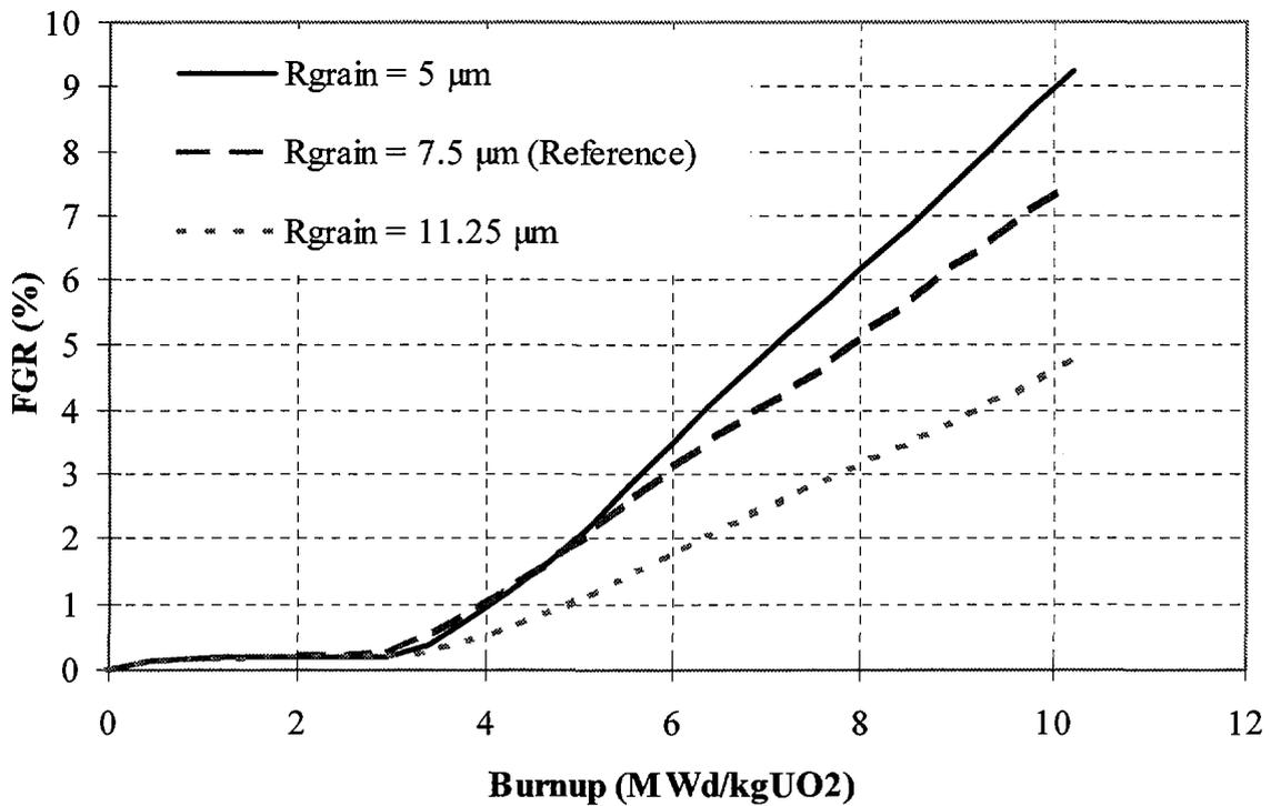
FIG. 4: The fission gas release rate at 38 kW/m as a function of the average burnup for three different average grain radii.
