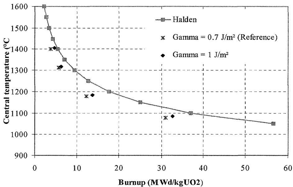
FIG. 2: The effect of the surface energy of intergranular bubbles (gamma) on the central temperature for 1% average fission gas release versus burnup during irradiation at constant linear heat rate.
