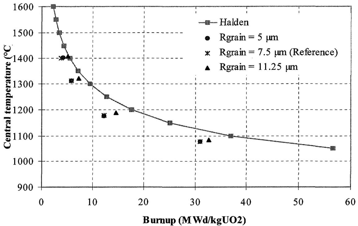
FIG. 3: The effect of the average grain radius on the central temperature for 1% average fission gas release versus burnup during irradiation at constant linear heat rate.
