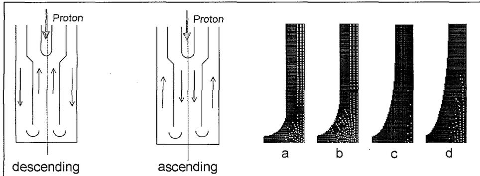
Figure 5: Types of PbBi flows inside the spallation module and types of window profiles (a=hemispheric).
