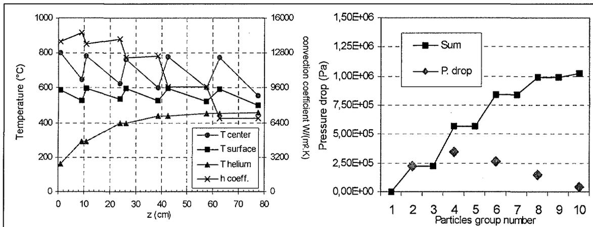
Figure 10: Temperature and pressure drop for a target with particles of increasing diameter.
