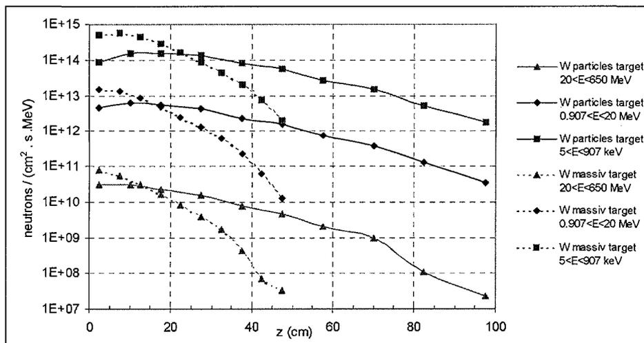
Figure 11: neutrons current density in both concepts of spallation targets.
