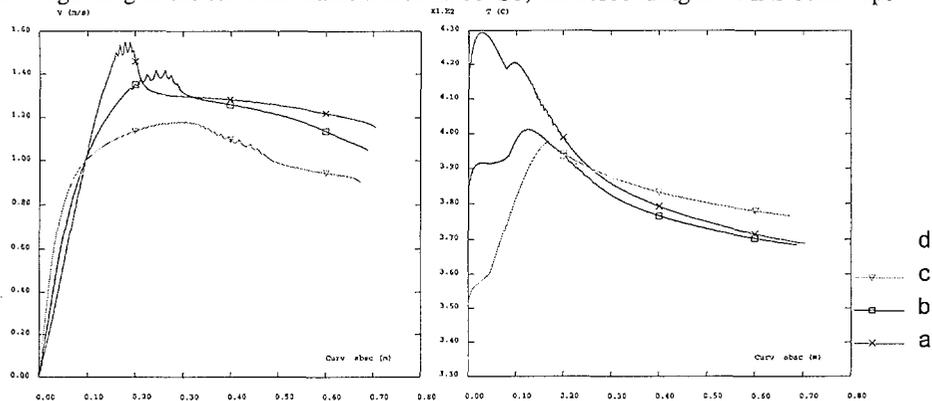
Figure 6: Velocity and temperature along the window for the different profiles, for  $V_e=1\text{m/s}$  and  $T_e=175^\circ\text{C}$ .
