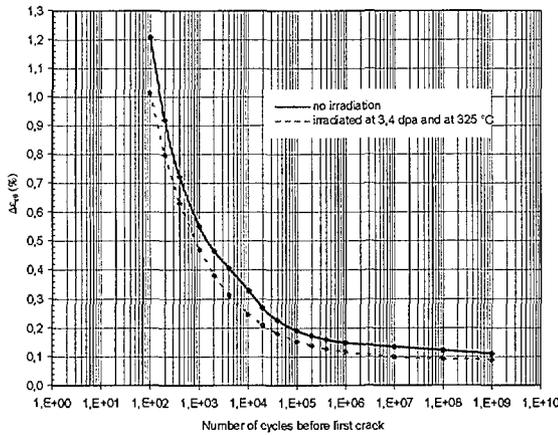
Figure 8: Fatigue curves of T91.
