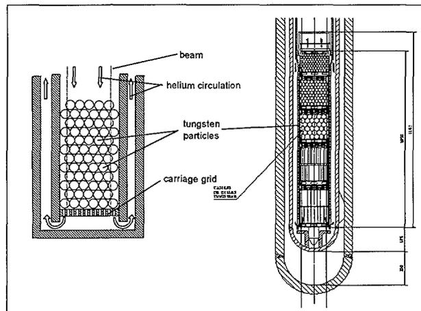
Figure 9: The CEA tungsten solid spallation target.
