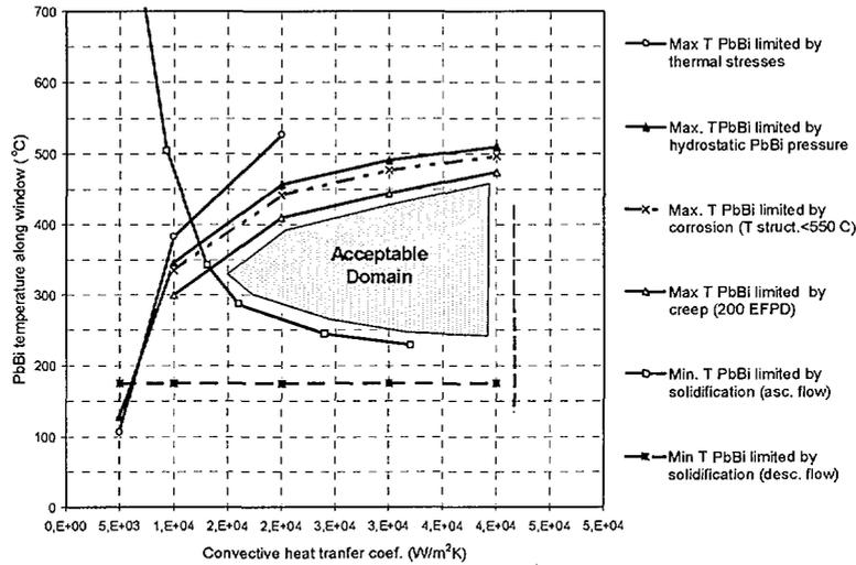
Figure 7: Acceptable operating range for the thermal-hydraulic parameters ( $T_{\text{PbBi}}$ ,  $h$ ) defining the cooling conditions along the window ( $E_p = 1.2$  GeV,  $I = 30$  mA,  $R_b = 13$  cm, PbBi pressure on window = 10 bar).
