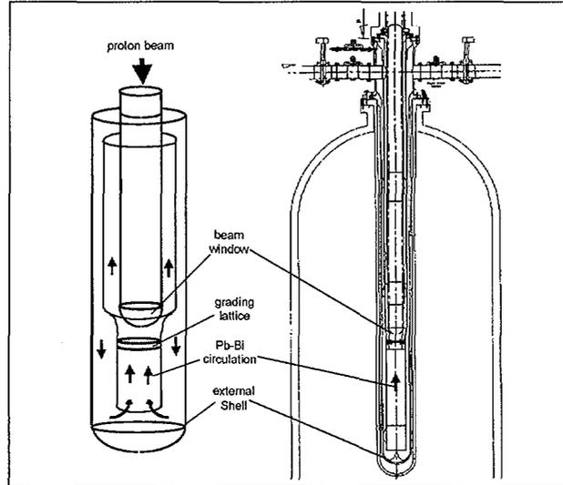
Figure 2: The CEA lead-bismuth liquid target.
