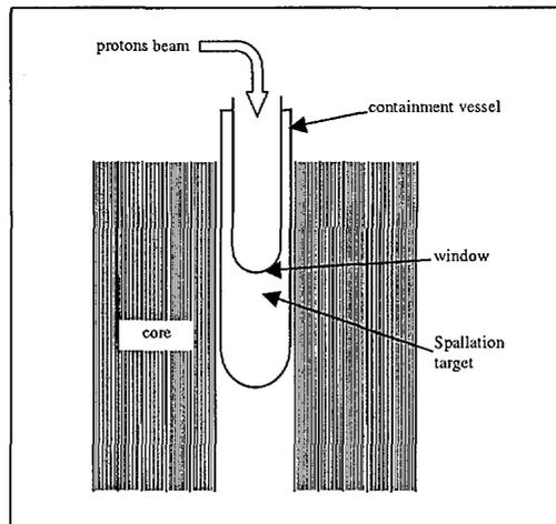
Figure 1: the spallation module in the middle of the core.
