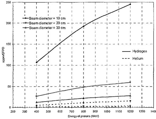
Fig. 4 shows that hydrogen is produced about 20 times more than helium. Hydrogen will diffuse in steel and be responsible of embrittlement while helium will entail swelling of the window. Between 400 and 1200 MeV, the former increases 15% and the latter increases less than 40%. As a result, gas production depends mainly on the current density, which is the key parameter.
