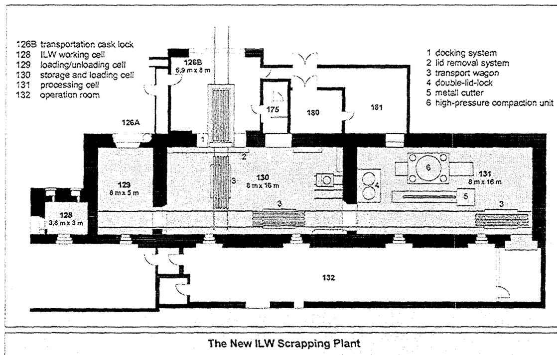
Fig. 1: Schema of the ILW scrapping facility
