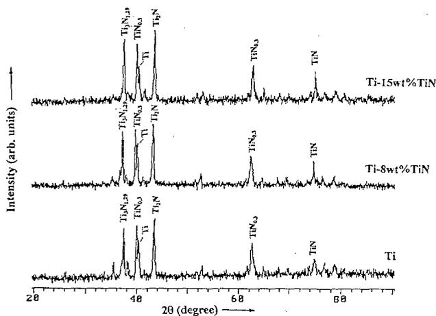
Figure 3: XRD pattern of pure Ti, Ti-8wt%TiN and Ti-15wt%TiN samples sintered at 1000°C in nitrogen atmosphere.
