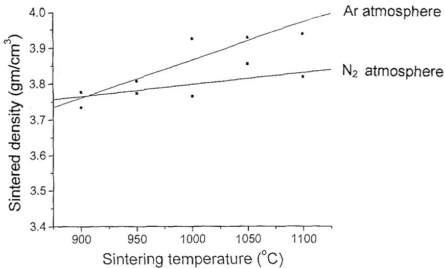
Figure 2©: Variation of sintered density as a function of sintering temperature for Ti-15wt%TiN samples sintered in argon and nitrogen atmosphere.
