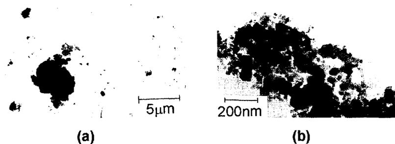
Figure 1: TEM photographs of (a) pure Ti powder and (b) TiN powder.
