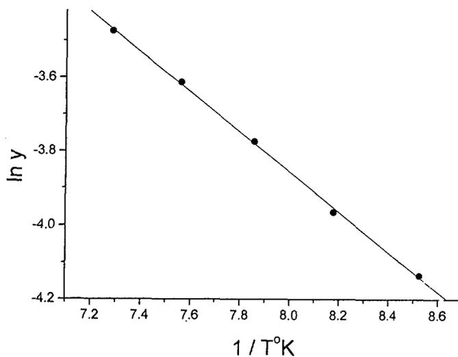
Figure 4(b): Arrhenius plot of pure Ti sintered in nitrogen atmosphere.
