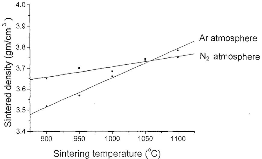
Figure 2(a): Variation of sintered density as a function of sintering temperature for pure titanium samples sintered in argon and nitrogen atmosphere.
