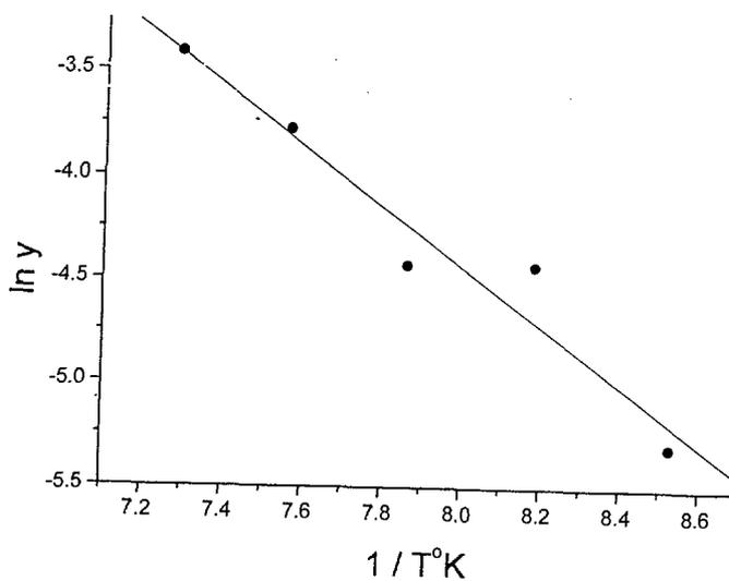
Figure 4(a): Arrhenius plot of pure Ti sintered in argon atmosphere.
