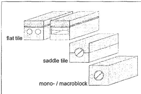
fig. 1: basic designs of high heat flux components for divertors
