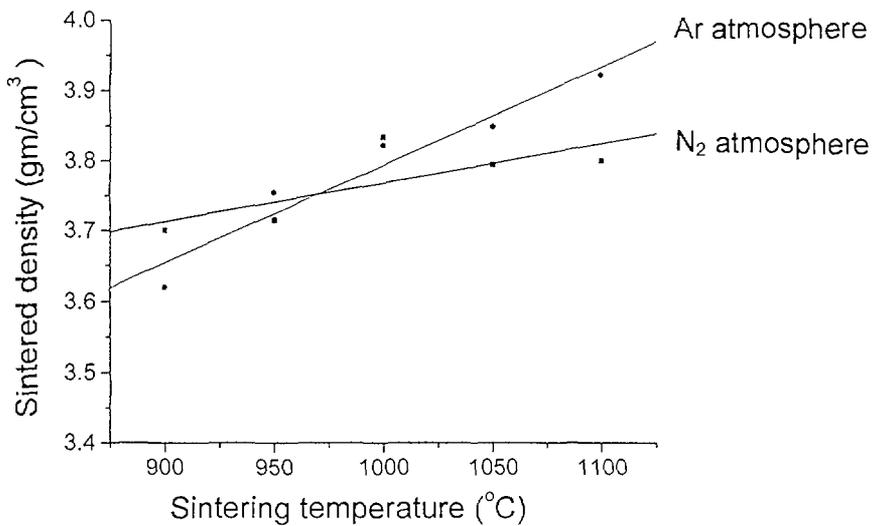
Figure 2(b): Variation of sintered density as a function of sintering temperature for Ti-8wt%TiN samples sintered in argon and nitrogen atmosphere.
