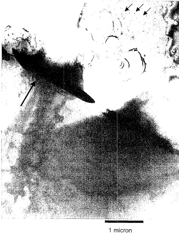
Figure 3. Large arrow indicates typical grain boundary carbide in stress-relieved TZM and the small arrows show typical matrix precipitate morphology.
