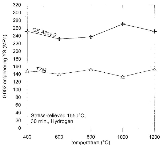
Figure 8. Yield strength of TZM and Alloy 2 after 1550°C heat treatment.
