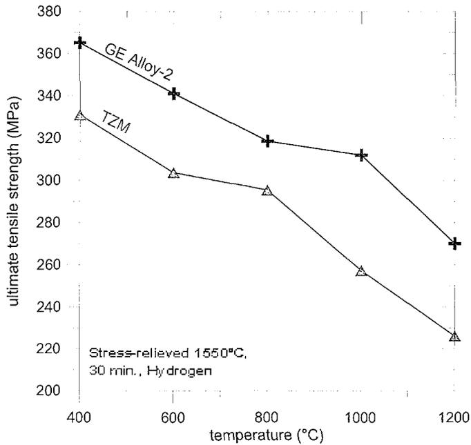
Figure 9. Ultimate strength after 1550°C heat treatment
