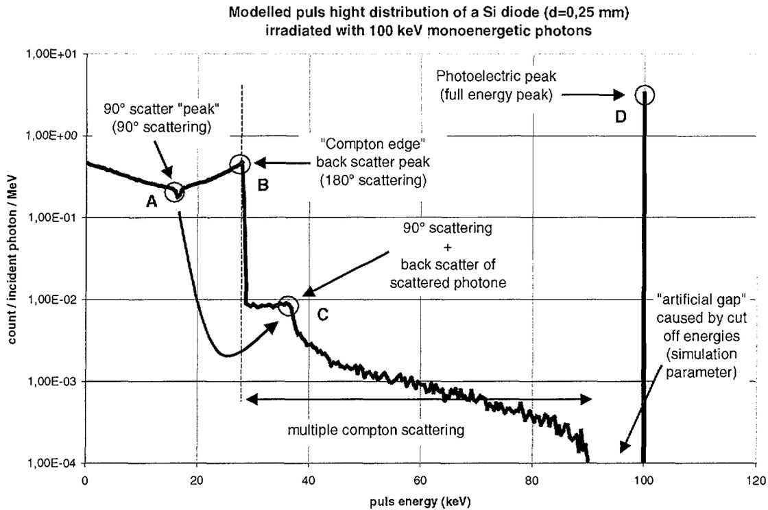
Figure 5 Simulated pulse height distribution in a 250µm thick Si diode. All peaks and edges are commented according their origin
