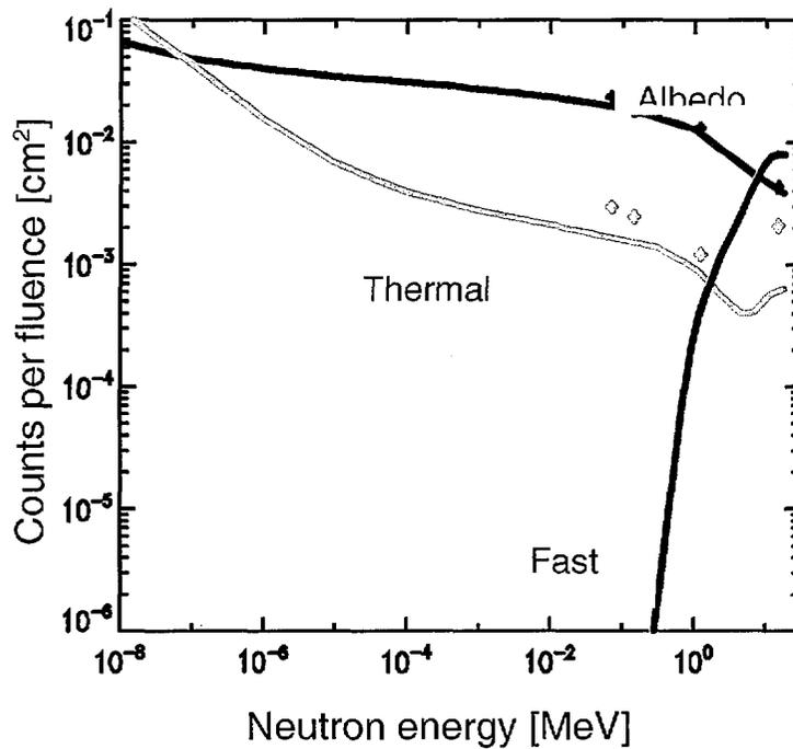
Figure 2 Theoretical modeling and experimental response for three types of sensors: two with  ${}^6\text{LiF}$  converter (front and back) for thermal neutrons and one with polyethylene converter (front) for fast neutrons
