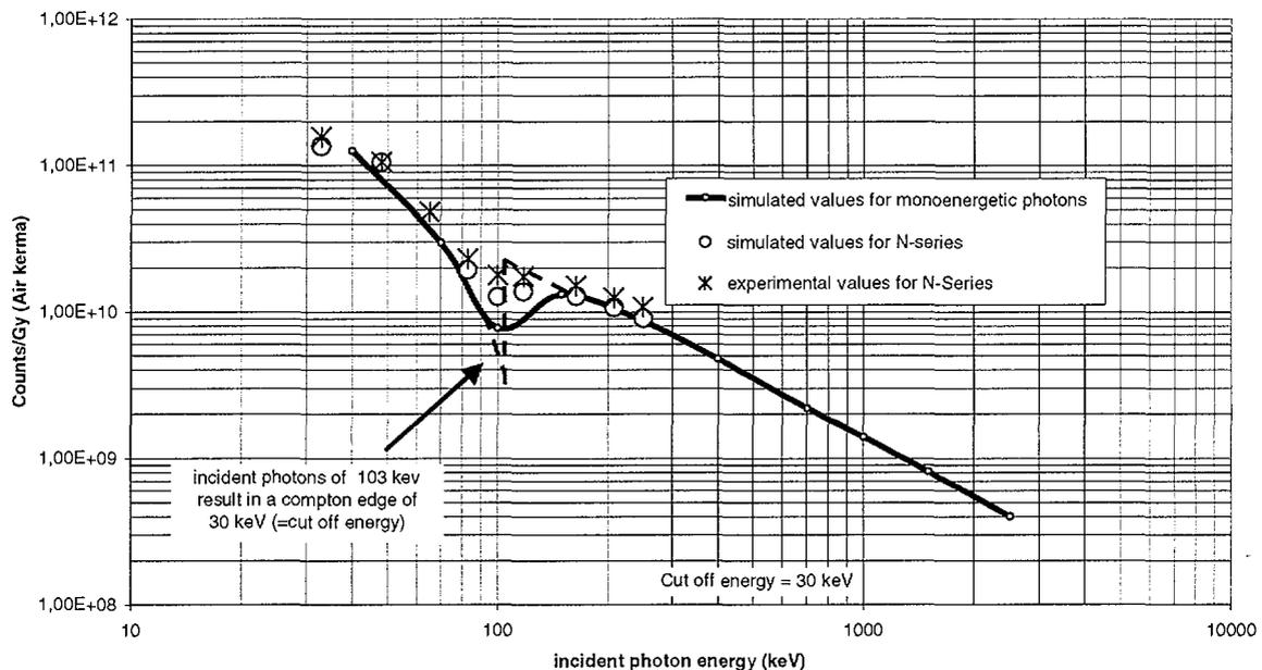
Figure 6 Comparison between simulation and experiment for a 250  $\mu\text{m}$  Si diode without a phantom for the total count response. Good agreement for low energy photons. At photon energies higher than 70 keV the experiments show higher values by a factor of 1,2
