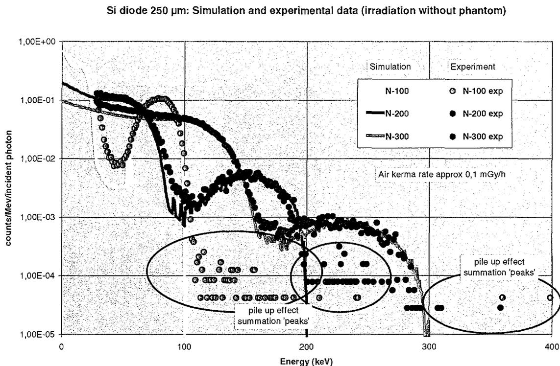
Figure 4 Comparison between Simulation and experiment for a 250  $\mu\text{m}$  Si diode without a Phantom. Good agreement in the photo peak region and in the compton region.
