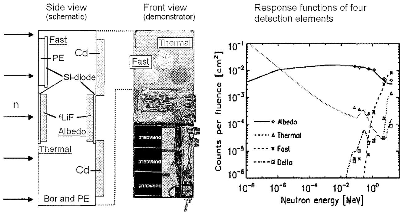
Figure 3 Integrated detector, schematically, photo and response function for three detectors: albedo fast and thermal
