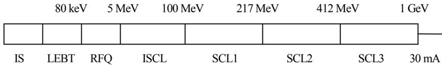
Fig. 1 The block diagram of the ADS accelerator
