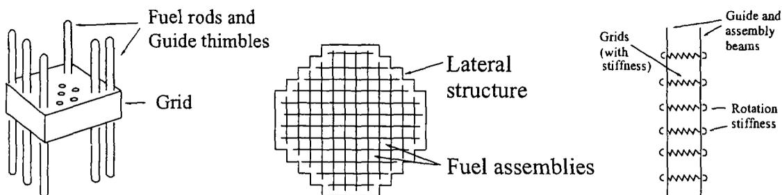
Figure 1: Fuel assembly, reactor core, and two-beam model
