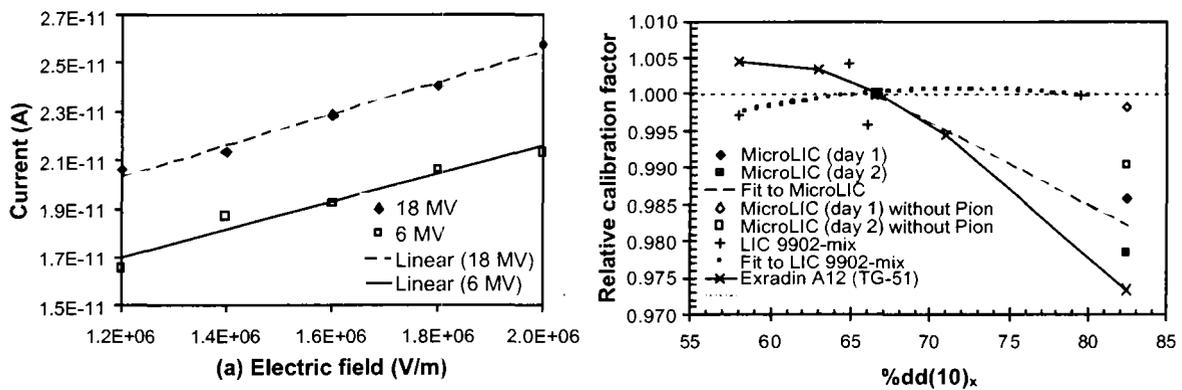
Fig. 1. (a) MicroLIC current as a function of applied electric field for 6 MV and 18 MV photon beams. (b) Relative calibration factor as a function of beam quality for the MicroLIC, LIC9902-mix [3] and Exradin A12 [1] chambers normalized to the response for the 6 MV photon beam. MicroLIC measurements from two days are shown both with (filled symbols) and without (open symbols) the ion recombination correction applied.
