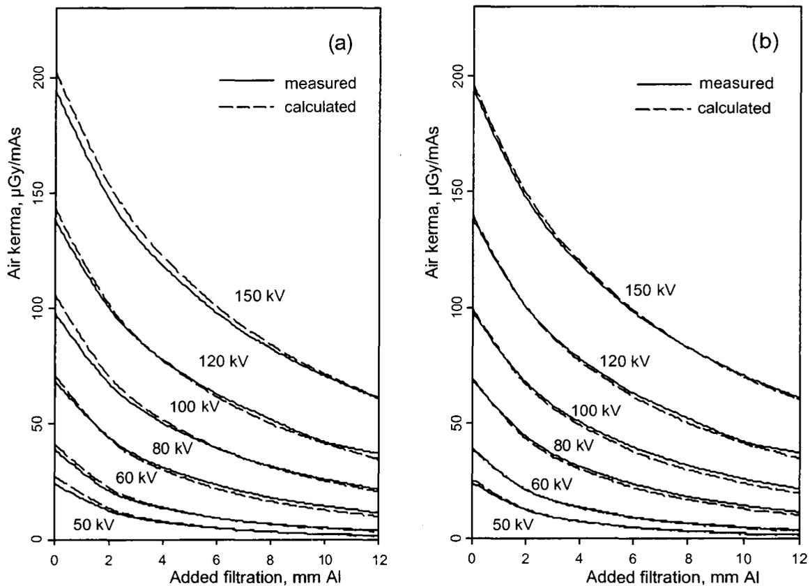
FIG. 1: Measured attenuation curves for various tube voltages obtained with an x-ray unit with  $16^\circ$  anode tube angle, 3.4% voltage ripple and 2.5 mm Al nominal inherent filtration in 100 cm distance: (a) data calculated with the same parameters but 3.12 mm Al inherent filtration, (b) data calculated with 2.5 mm Al inherent filtration plus an additional filter of  $6.37 \mu\text{m W}$ .
