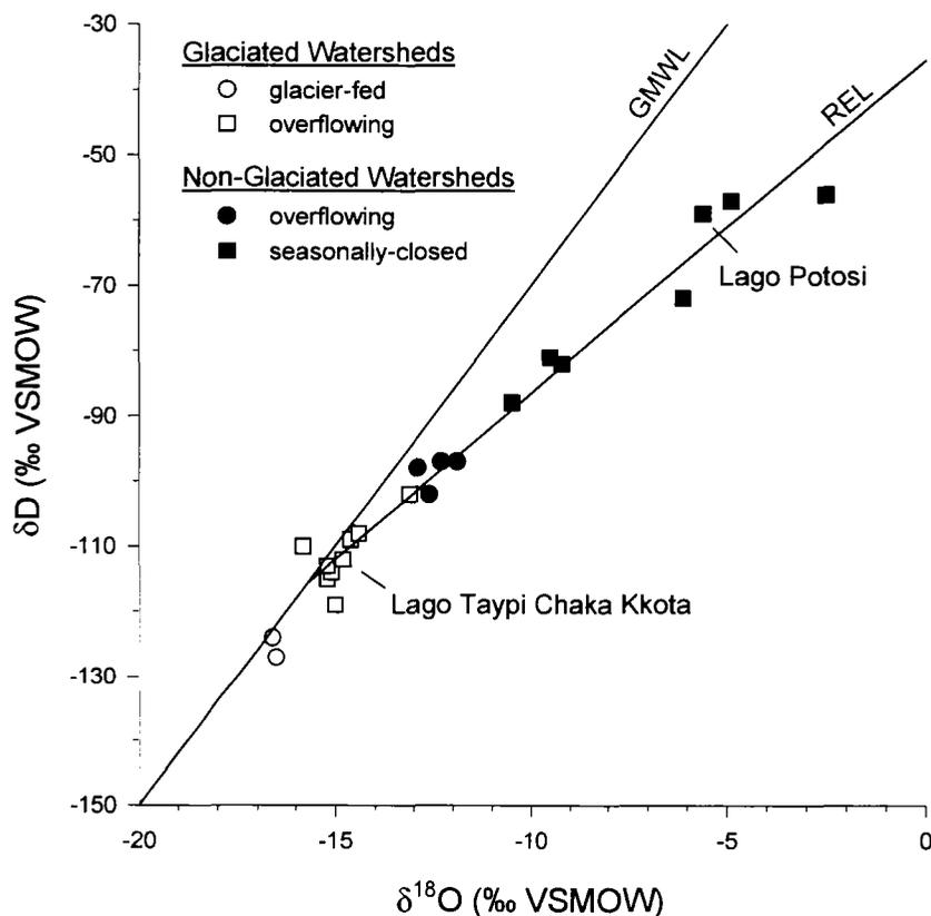
FIG.1. Isotopic composition of lake waters from the Bolivian Andes sampled in June 1997 [10]. Also shown are the Global Meteoric Water Line (GMWL:  $\delta\text{D} = 8 \delta^{18}\text{O} + 10$ ) and the Regional Evaporation Line (REL:  $\delta\text{D} = 5.1 \delta^{18}\text{O} - 35.5$ ).
