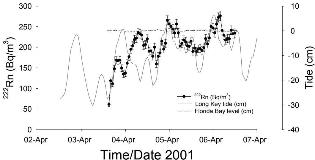
Figure 1 Concentrations of  $^{222}\text{Rn}$  in Florida Bay waters off Key Largo (left-hand scale) and the water levels in Florida Bay and the Atlantic (right-hand scale). The rhythmic pattern of  $^{222}\text{Rn}$  is responding to tidal forcing on the opposite (ocean) side of the island that drives subsurface waters into Florida Bay.
