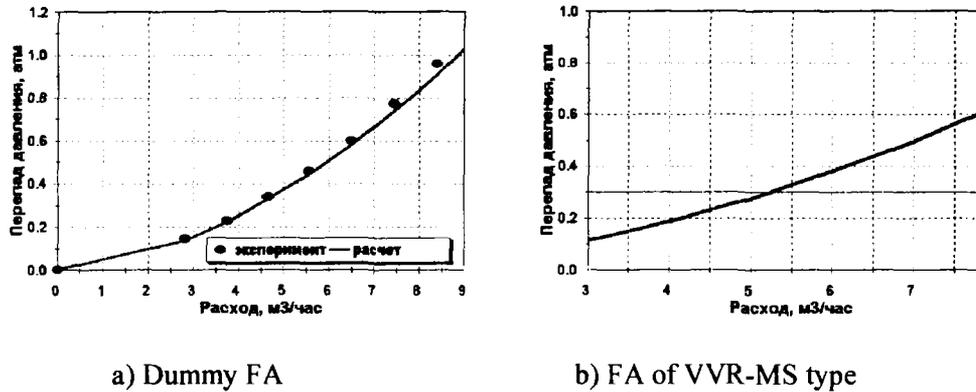
Fig.3. Pressure fall vs. consumption
