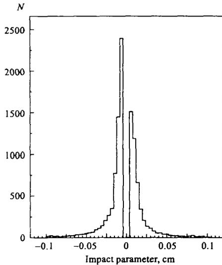
Fig. 9. Impact parameter distribution for tracks which pass the online cuts (number of tracks  $\geq 2$ ,  $\chi^2 < 25$ ,  $P_T > 2 \text{ GeV}/c$ , and  $50 \mu\text{m} < d < 0.1 \text{ cm}$ )
