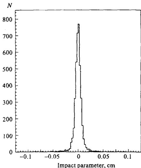
Fig. 6. Impact parameter distribution for data taken in October, 2001, for track candidates with  $\chi^2 < 10$  and  $P_T > 2$  GeV/c, after correction for beam position offset, relative misalignment of the wedges and nonlinearity. In this case the correction for the beam tilt was not necessary since the tilt was  $\simeq 0$ . The Gaussian fit gives  $\sigma = 48 \mu\text{m}$
