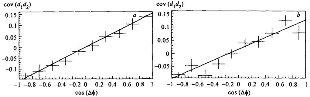
Fig. 8. Covariance of the two impact parameters of track pair versus the cosine of the difference of the two azimuthal angles: when the beam tilt is  $\simeq 800 \mu\text{rad}$  (a) and  $\simeq 0$  (b)
