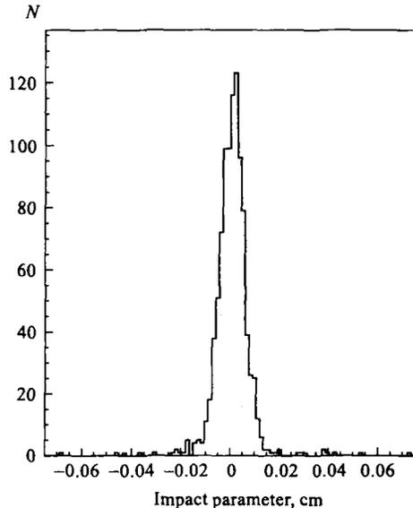
Fig. 7. Impact parameter distribution for the October, 2000 Commissioning Run data, after all the cuts and correction. The Gaussian fit gives  $\sigma = 45 \mu\text{m}$
