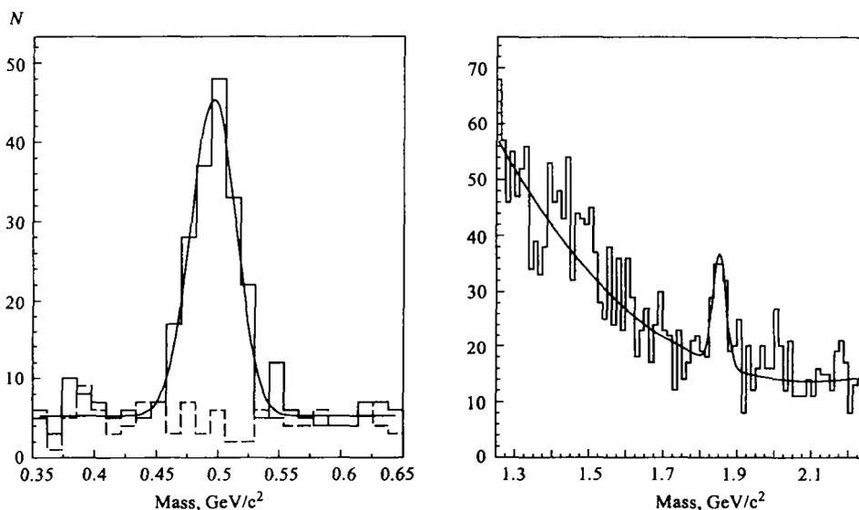
Fig. 10. Invariant mass distribution for track pairs, assuming the two tracks to be  $\pi^+$  and  $\pi^-$
