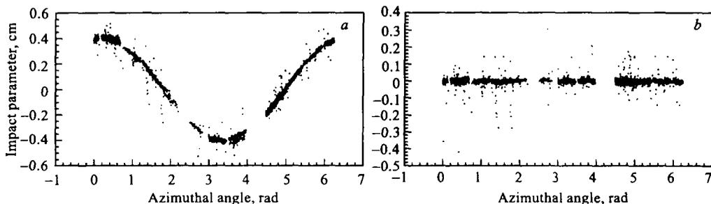
Fig. 4. Impact parameter versus azimuthal angle for candidate tracks with  $\chi^2 < 10$  in the standard configuration before (a) and after beam offset correction (b)
